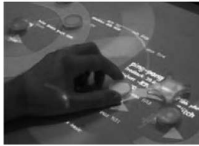
PHOTO 21.4 AudioPad running on Sensetable platform. Audiopad is a composition and performance environment for electronic music. Tangibles are tracked on an interactive tabletop system; their evolving physical/digital state is transformed into music.
