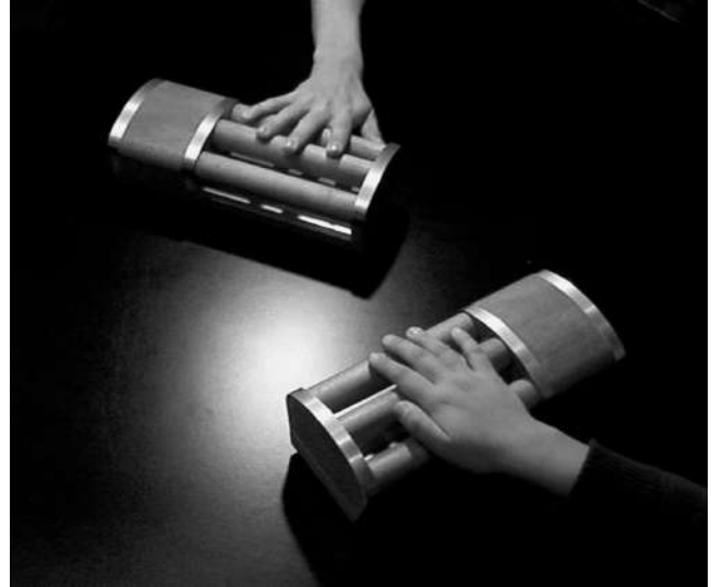
PHOTO 21.3 inTouch. inTouch is a prototype that explores tangible telepresence using touch over distance. Key idea is synchronizing distributed physical objects using force feedback technology.
