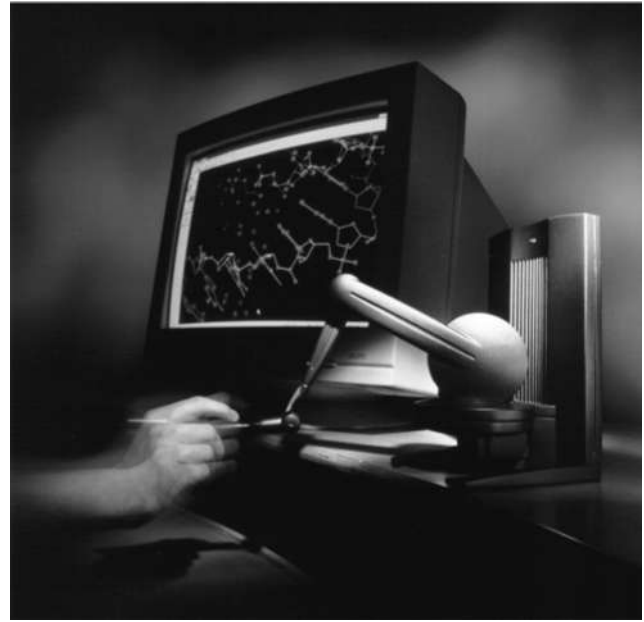
FIGURE 9.3 PHANToM, one of the most popular commercially available haptic interfaces.
