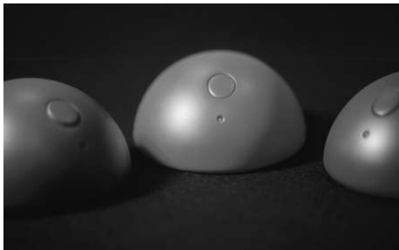
PHOTO 21.9 Curlybot. Curlybot is a toy that records and plays back physical motion. Curlybot remembers how it has been moved by human users, and can replay this movement with all the intricacies of the original gesture. Every pause and acceleration – even shaking in users’ hands – is recorded and repeatedly relived, allowing simple gestures to expand into complex geometric patterns.
