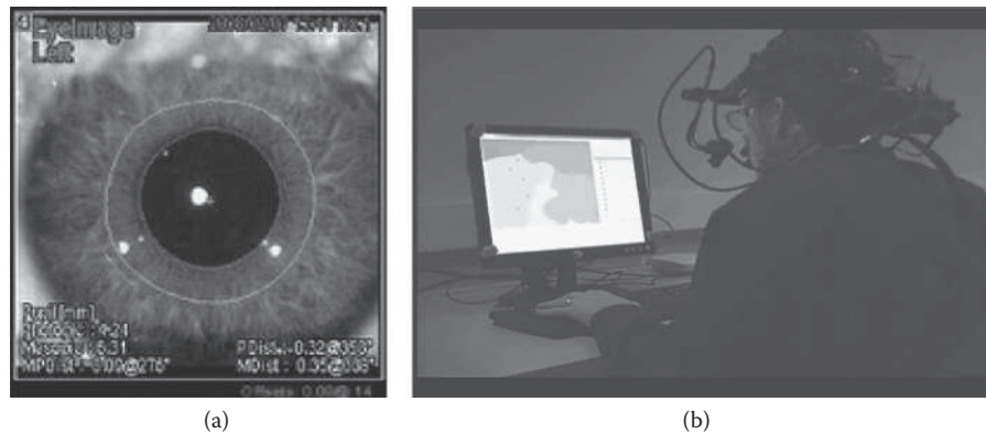
FIGURE 60.4 Equipment used to collect pupillometry data as part of Lockheed Martin Advanced Technology Laboratory's AugCog system. (a) Pupillometry display. (b) Head-mounted hardware to capture pupil changes.
