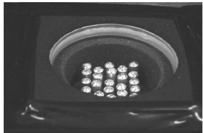
FIGURE 9.13 Top end of the rods conforming haptic surface.
