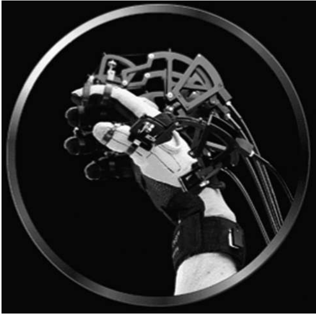
FIGURE 9.2 CyberGrasp, a commercially available exoskeleton in which cables are used to transmit force.
