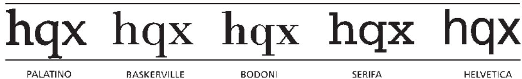
FIGURE 14.17 Black on white versus white on black. The x-height of a typeface (based on the actual height of a lowercase x) is a key characteristic when deciding the visual size of a typeface, particularly when readability is critical. While the above typefaces are the same point size, some seem larger (e.g., Helvetica) and easier to read than others (e.g., Serifa). Letterforms often appear as black/dark shapes on white/light backgrounds. The eye also reads the reverse, or negative shape around a letterform, which can create a shape that visually distracts and makes text difficult to read. Try setting a paragraph of black type on a white background, then set the same exact paragraph with white type on a black background. You can also try this same exercise with a dark color on a light background, and then try the reverse. You will notice that the greater the contrast (e.g. white type on black) the harder it is to read in large amounts.
