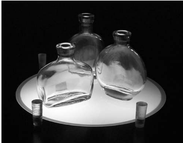
PHOTO 21.8 musicBottles. musicBottles is a tangible interface in which bottles exist as containers and controls for digital information. The system includes a specially designed table and (here) three corked bottles that “contain” the sounds of classical, jazz, and techno music. The interface allows users to structure the experience of the musical composition by physically manipulating the different sound tracks.
