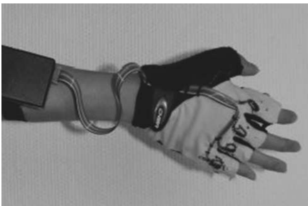
FIGURE 12.22 The Mobile Music Touch glove allows users to learn note sequences while performing other tasks.
