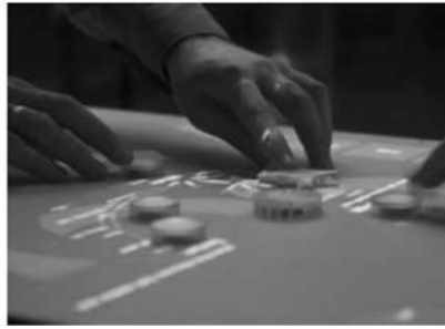
PHOTO 21.4 AudioPad running on Sensetable platform. Audiopad is a composition and performance environment for electronic music. Tangibles are tracked on an interactive tabletop system; their evolving physical/digital state is transformed into music.
