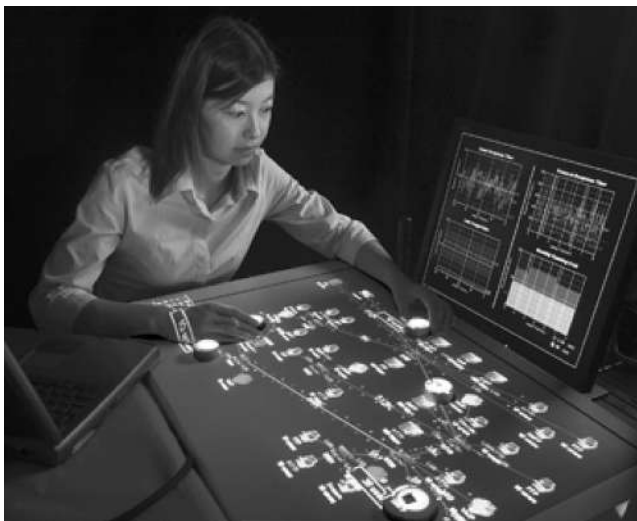
PHOTO 21.5 IP Network Design Workbench running on Sensitable platform. The IP Network Design Workbench supports collaborative network design and simulation by multiple experts and customers on the Sensetable platform using an event-driven simulation engine.
