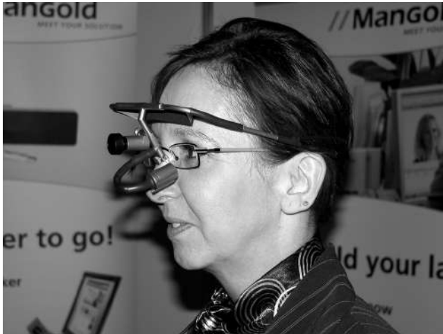
FIGURE 15.4 Example of a head-mounted display for conducting eye tracking of users during testing of mobile-phone applications. The unit is attached to a small portable device that the user carries. (Courtesy of Mangold International, Arnstorf, Germany).
