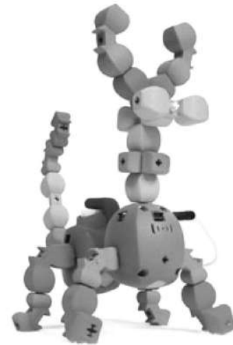
PHOTO 21.10 Topobo. Topobo is a 3D constructive assembly system with kinetic memory: the ability to record and play back physical motion. Topobo is distinguished by its coincident physical input and output behaviors.
