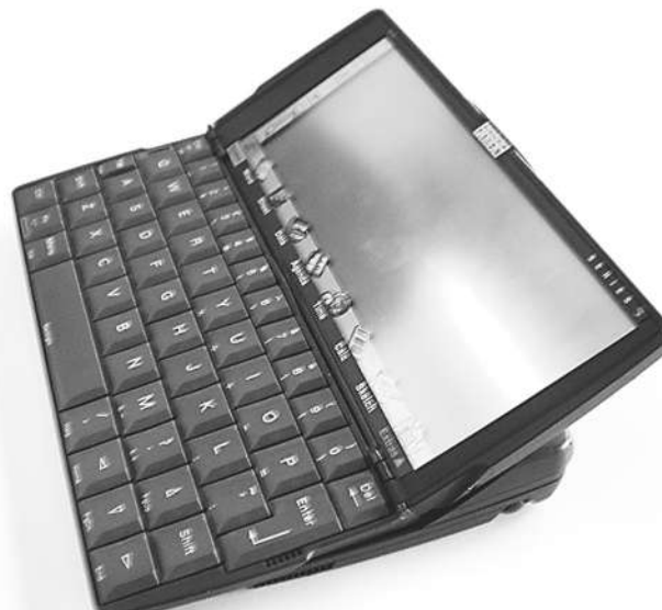
FIGURE 6.9 The Psion Series 5 handheld device, circa 1995. The resistive touch screen supports stylus or touch input. Note the counterweight on the bottom part of the clamshell that prevents the device from tipping over when one interacts with the screen.
