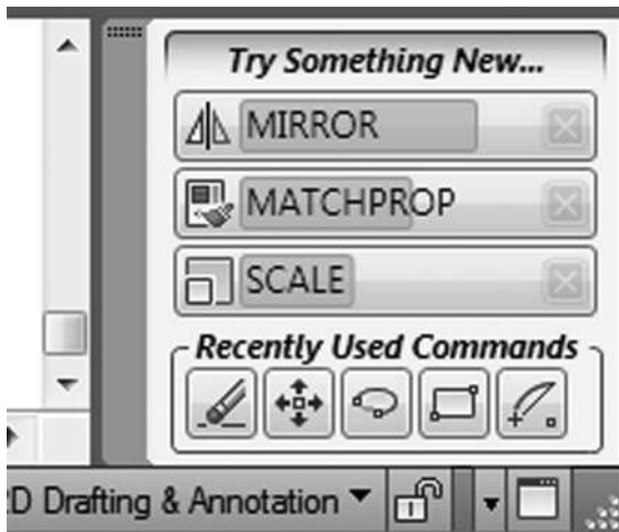
FIGURE 19.1 Screenshot showing how COMMUNITYCOMMANDS recommends commands to a user. (Image supplied by Justin Matejka. The length of the darker bar for a command reflects its estimated relevance to the user’s activities. When the user hovers over a command in this interface, a tooltip appears that explains the command and might show usage hints provided by colleagues. See also http://www.autodesk.com/research .)
