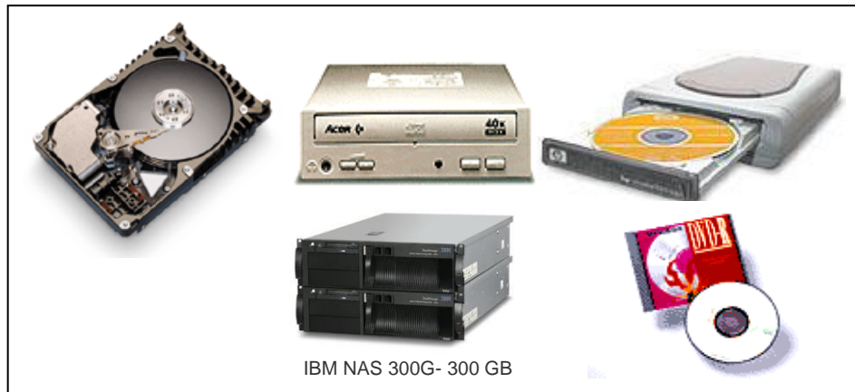
Gambar 8.9 Hardisk, NAS 300G, Driver CD ROM/RW (650MB), DVD ROM/RW (4.7-50 GB), C/DVD R/RW
