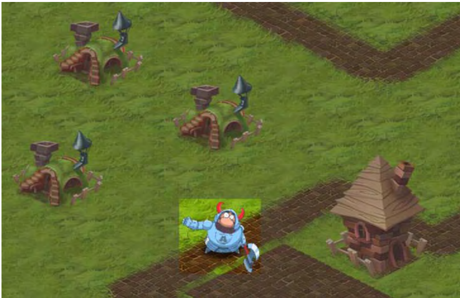
Figure 7-20. The area that changes between frames is much smaller than the screen; still, we repaint it all on every frame.
