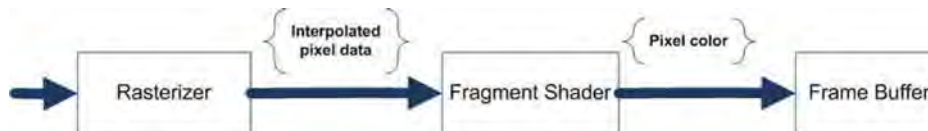
Figure 9-3. In the second part of rendering process, data received from the vertex shader is interpolated and passed to the fragment shader. The fragment shader outputs the pixel color.
