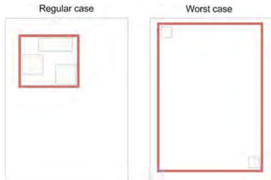
Figure 7-22. We have a small dirty rectangle in a regular case, but the worst case results in repainting the entire area.
