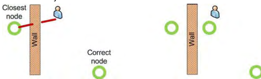
Figure 13-13. On the left, the problem with a naive pathfinding graph: due to the mistake of the level designer, the character attempts to move through the wall to reach the node. The corrected version is on the right.
