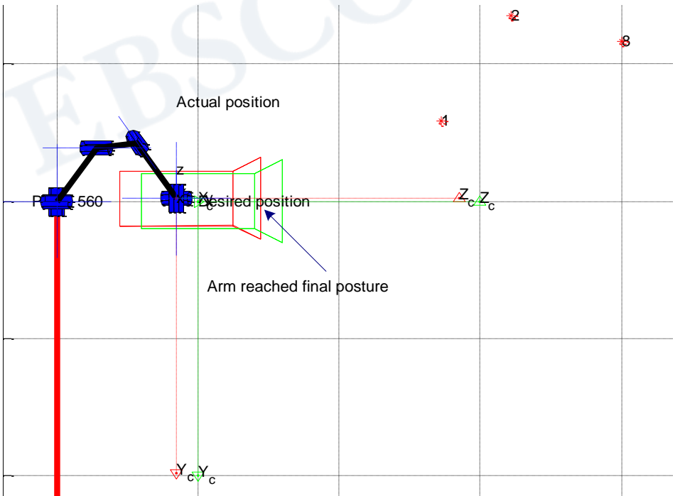
Figure 10. Robot arm-camera servoing towards a desired object posture.
