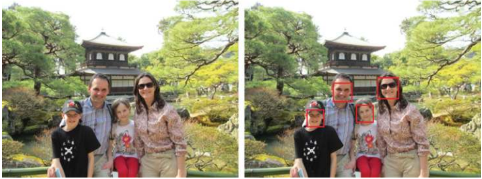
Figure 8.20 Face recognition using the cascade of Haar classifiers. Note that this recognition is performed on a grey-scale version of the image and is capable of dealing with faces of different sizes
