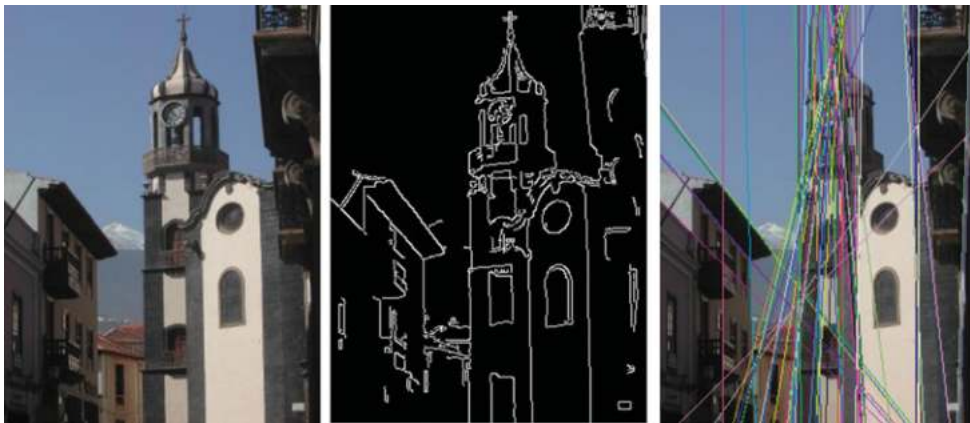
Figure 6.26 The Hough transform for straight lines. The original image (left), edges computed using the Canny operator (centre) and the located edges (right)
