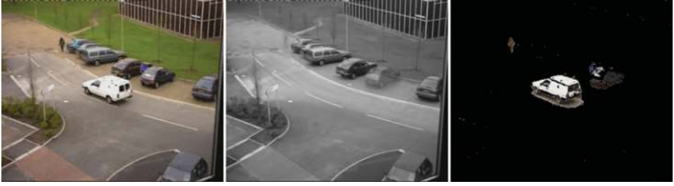
Figure 9.8 The current frame (left), the running average with selective update background image with \alpha = 0.01 for background points and \alpha = 0.0033 for background points (centre), the detected moving pixels image (right). Compared to Figure 9.7 we can see that the car on the road on the right of the image has been effectively averaged out of the background, and that the car which parked is slowly being averaged into the background. Note that the background model is a grey-scale image. A colour version of this model is provided in the resources accompanying the text. The original images are from the PETS 2000 dataset. Reproduced by permission of Dr. James Ferryman, University of Reading
