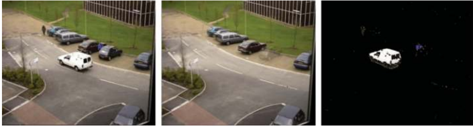
Figure 9.10 Current frame from a video sequence (left) together with a weighted image of the GMM background, where the weight of each Gaussian defines how the averages of the Gaussians are combined (centre) and the detected moving object pixels (right). The moving objects from the first frame (see Figure 9.3) have been removed and the parked car has been incorporated into the background. The original images are from the PETS 2000 dataset. Reproduced by permission of Dr. James Ferryman, University of Reading
