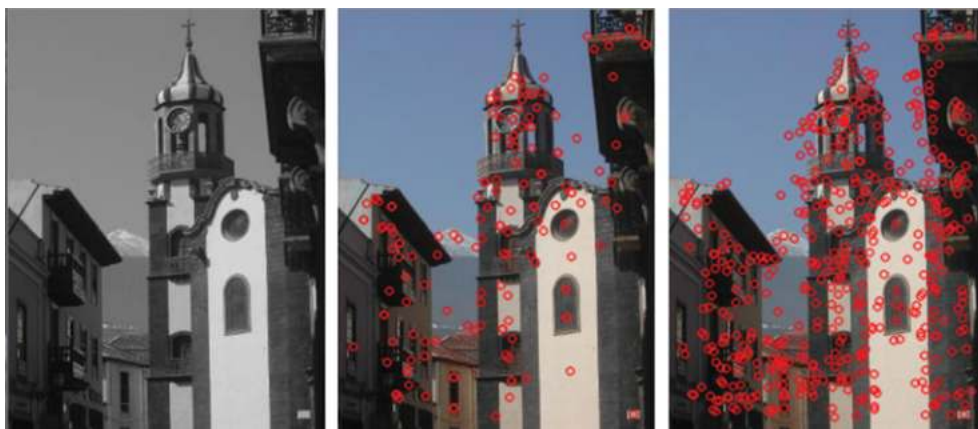
Figure 7.18 SIFT features (centre) and SURF features (right) as derived from the grey-scale image on the left
