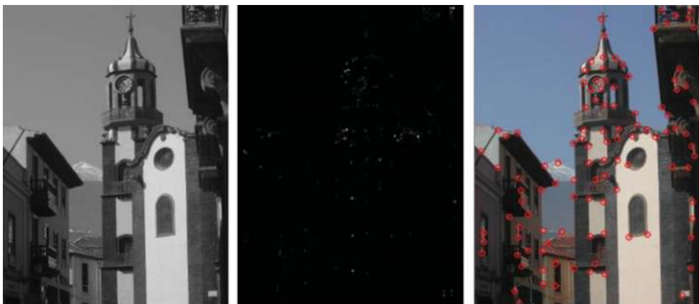
Figure 7.7 The Harris/Plessey corner detector. The grey-scale image (left) was processed to obtain the cornerness map (centre) which in turn was analysed to extract the corners (right)
