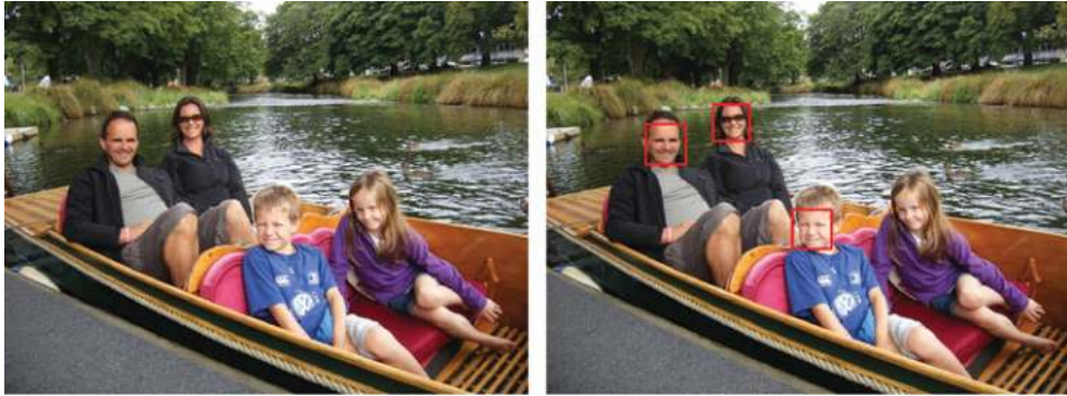
Figure 8.24 Face recognition using the technique described in this chapter. Note that recognition has failed on one of the faces. This is most probably due to the angle of the face (i.e. it is not full frontal)
