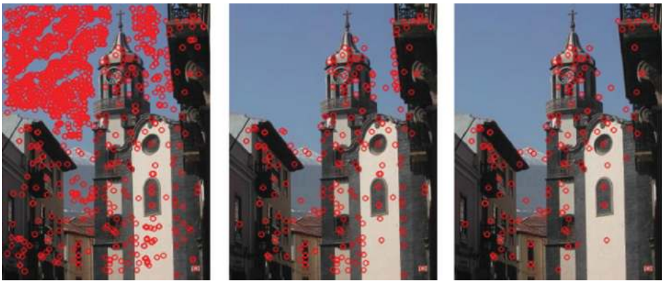
Figure 7.14 Scale invariant keypoints (left), after discarding low contrast keypoints (centre) and after discarding poorly localized keypoints (right)
