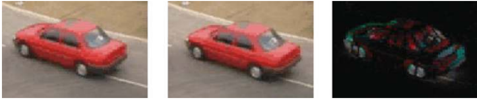
Figure 9.4 The current frame (left), the previous frame (centre), and the difference image (right). The original images are from the PETS 2000 dataset. Reproduced by permission of Dr. James Ferryman, University of Reading
