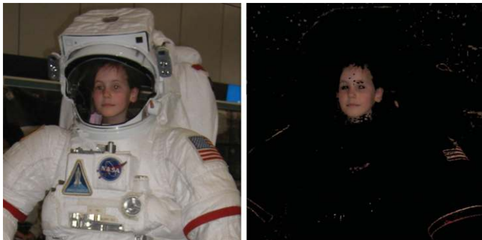
Figure 2.12 Colour image (left), selection of skin pixels by selecting all points with (Saturation \geq 0.2 ) AND ( 0.5 < \text{Luminance}/\text{Saturation} < 3.0 ) AND ( \text{Hue} \leq 28^\circ OR \text{Hue} \geq 330^\circ ) (right)
