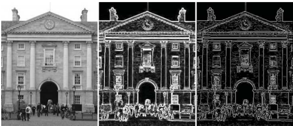
Figure 6.9 An image (left) together with the derived gradients (centre) and the non-maxima suppressed gradients (right)
