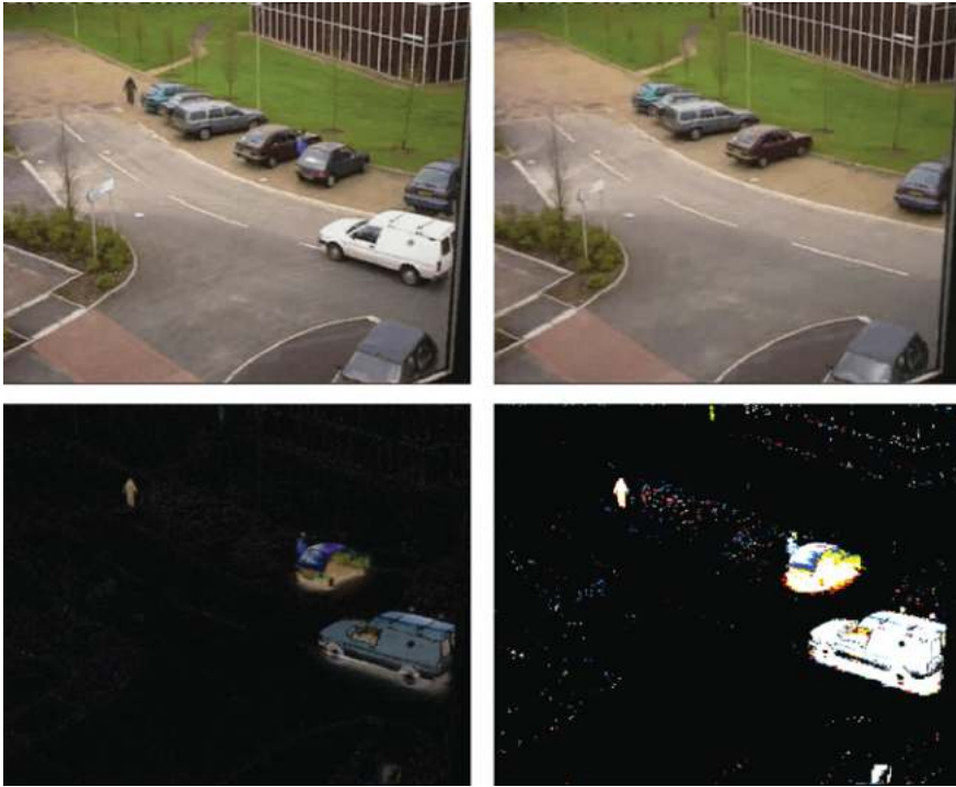
Figure 9.1 The current frame of a video sequence (top left), the background image (top right), the colour difference image where the difference for each channel has been computed separately (bottom left) and a thresholded version of the difference image (bottom right) again processed on a per channel basis. The original images are reproduced by permission of Dr. James Ferryman, University of Reading
