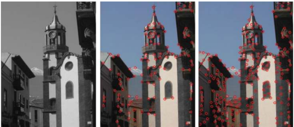
Figure 7.17 Harris features (centre) and minimum eigenvalue features (right) as derived from the grey-scale image on the left
