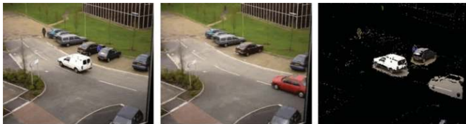
Figure 9.3 The current frame (left), the static background image (centre), the detected moving pixels image (right). The background image contains some moving objects (the red car and the person at the top of the image), and the corresponding pixels are identified as being moving pixels in the current frame. In addition, the car which has parked since the start of the video has not been included in the background and hence is still identified as moving. The original images are from the PETS 2000 dataset. Reproduced by permission of Dr. James Ferryman, University of Reading
