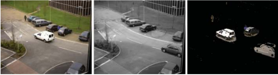
Figure 9.7 The current frame (left), the running average with selective update background image with \alpha = 0.01 (centre), the detected moving pixels image (right). The good news is that the blurred person (from Figure 9.3) has been removed from the background image. However, as the processing was started on the same frame as in the static background example (see Figure 9.3), it suffers from the same problems. The moving due to the selective update. In addition, the parked car has not been included in the background but the pixels around the car are updating, resulting in a halo effect around the position of the parked car in the background image. Note that the background model is a grey-scale image. A colour version of this model is provided in the resources accompanying the text. The original images are from the PETS 2000 dataset. Reproduced by permission of Dr. James Ferryman, University of Reading
