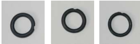
Figure 10.3 Sample images of good O-rings (i.e. with no defects; see top row), broken O-rings (middle row) and O-rings with notches out of them (bottom row)
