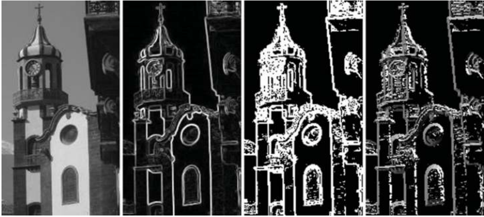
Figure 6.1 A grey-scale image of a church (left), the Sobel edge gradient magnitude (centre left), a thresholded version of the gradient magnitude (centre right) and the corresponding Sobel orientations (right)
