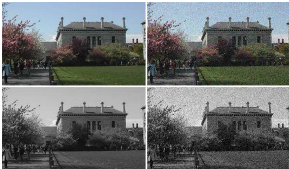
Figure 2.14 Colour and grey-scale images (left) with Gaussian noise added with a mean of 0 and a standard deviation of 20 (right). The signal to noise ratios of the noisy images are 43.3 (colour image) and 40.3 (grey-scale image), with respect to the original images
