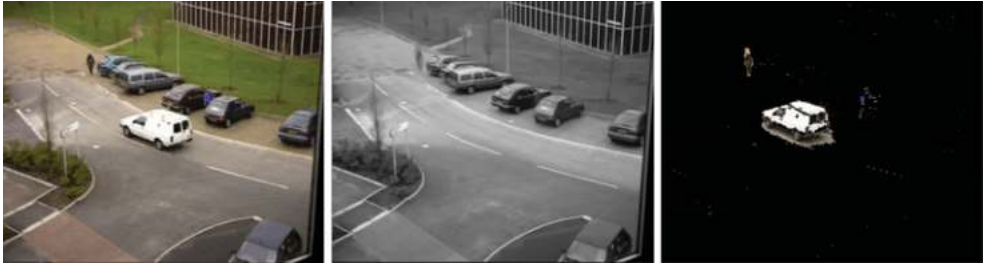
Figure 9.5 The current frame (left), the running average background image with \alpha = 0.01 (center), the detected moving pixels image (right). The processing was started on the same frame as in the static background example (see Figure 9.3), and it is notable that the moving objects from the start frame are no longer visible in the background image. In addition, the parked car has been incorporated into the background. The background image is contaminated by blurred versions of any moving objects. The person to the left of the parked cars is clearly visible in the background image. The white van is not particularly visible in the background image mainly due to the fact that it is just brightening the background somewhat. Note that the background model is a grey-scale image. A colour version of this model is provided in the resources accompanying the text. The original images are from the PETS 2000 dataset. Reproduced by permission of Dr. James Ferryman, University of Reading
