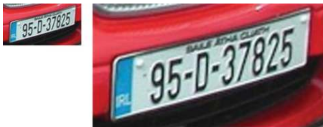
Figure 5.8 Bi-cubic interpolation when expanding an image 4-fold
