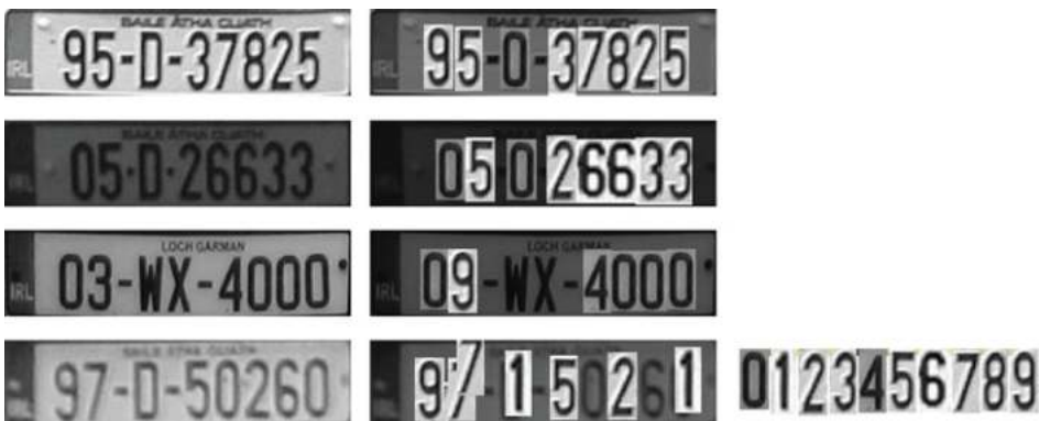
Figure 8.2 Recognition of license plates (original images are on the left, images with recognised characters overlaid are in the middle, and the templates used are on the right)
