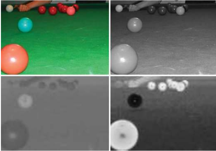
Figure 2.9 YUV image (top left) shown with luminance (Y) channel (top right), U channel (bottom left) and V channel (bottom right)
