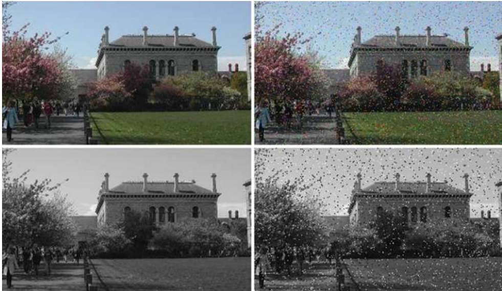
Figure 2.15 Colour and grey-scale images (left) with 10% Salt and pepper noise (right). The signal to noise ratio of the noisy images are 7.5 (colour image) and 6.7 (grey-scale image)
