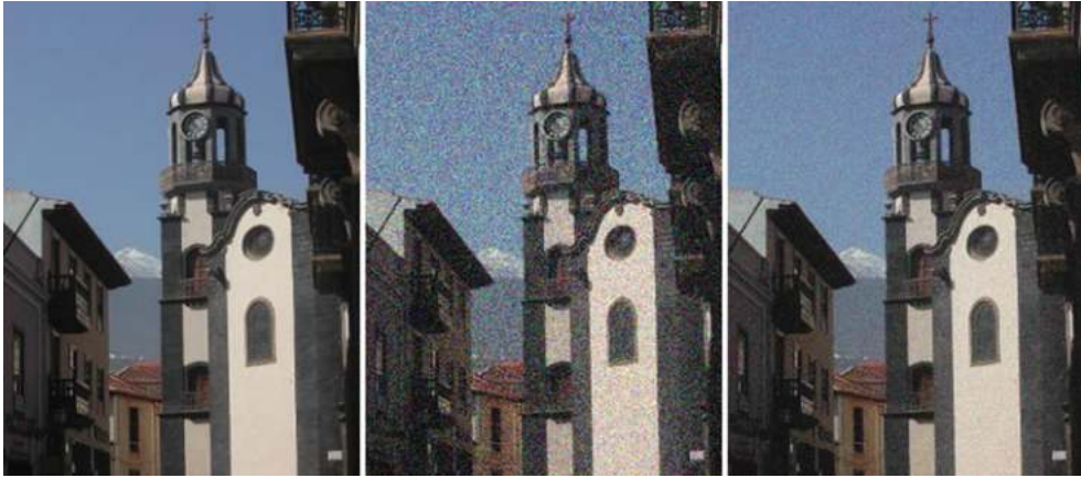
Figure 2.16 Original image (left), with Gaussian noise added (middle, 0 mean and 30 standard deviation) and the average of 8 such noisy images (right). Note how closely the final image approximates the first one. The signal-to-noise ratio in the middle image is 17.5, whereas it has increased to 129.7 in the averaged image
