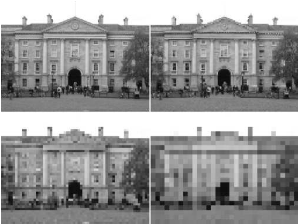
Figure 2.2 Four different samplings of the same image; top left 256x192, top right 128x96, bottom left 64x48 and bottom right 32x24
