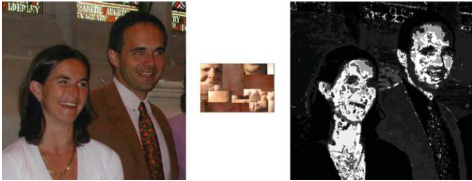
Figure 3.8 Back-projection (right image) of a (3D) HLS histogram of the skin pixels (centre image) of a colour image (left image). The 3D histogram was quantized to 3 bits per channel (i.e. the histogram was 8 \times 8 \times 8 ) and this histogram was normalised so that the maximum value was 1.0
