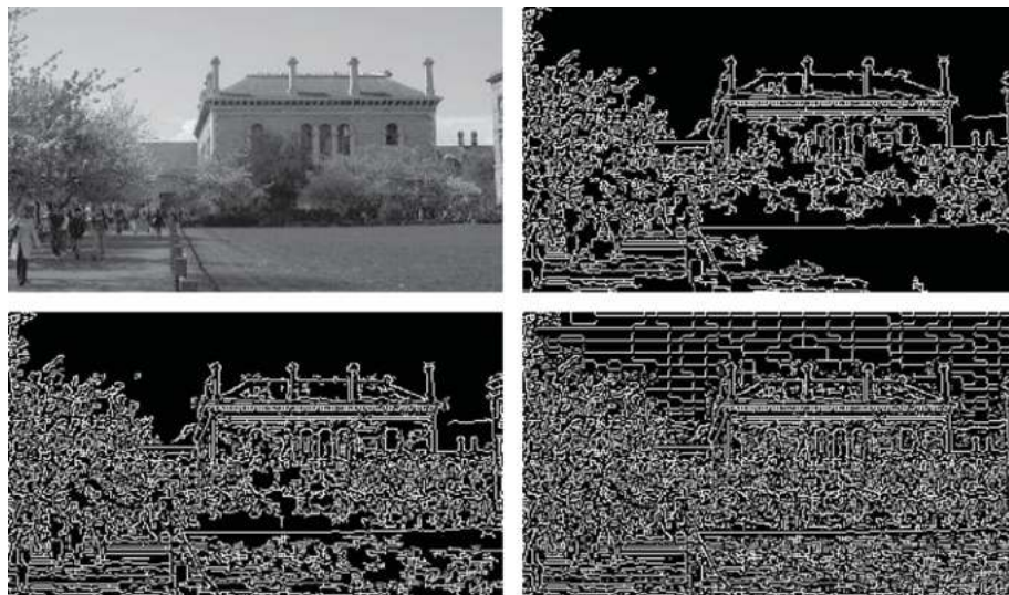
Figure 6.14 Canny edge detection. The three Canny images all use the same smoothing filter but various low and high gradient thresholds (7 and 236 – top right, 7 and 100 – bottom left, 1 and 1 – bottom right). The bottom right image shows all possible edges and the other two show some of the effects of the thresholds
