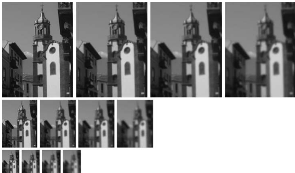
Figure 7.11 Scale images considered in the determination of SIFT features. Three octaves of scale space are shown where each octave corresponds to a doubling of the standard deviation ( \sigma ) which is applied to the left most image. The images in each octave are convolved with a number of Gaussians L_n(i, j, k, \sigma) = G(i, j, k^n \sigma) * f(i, j) where n = 0, 1, 2, 3, \dots
