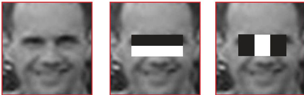
Figure 8.22 A sample face sub-image and the first two features used in the cascade of features for face recognition. These features seem to make logical sense, as the first appears to correspond to the notion that the cheek region will be brighter than the eye region and the second appears to indicate that the space between the eyes will be brighter than the eyes
