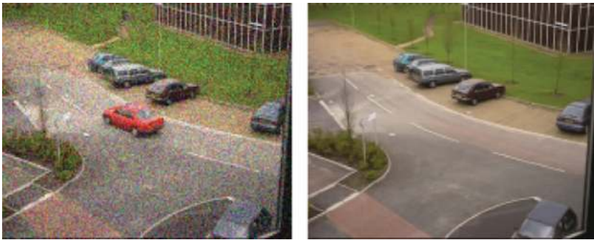
Figure 9.6 Current frame from a video sequence contaminated by significant Gaussian noise (left) together with the running average background (right) with w = 0.01 . While moving objects are incorporated somewhat (notice the red blurring on the road caused by the moving car) into the background, it is clear that the noise in the video is significantly reduced in the background image. The original images are from the PETS 2000 dataset. Reproduced by permission of Dr. James Ferryman, University of Reading
