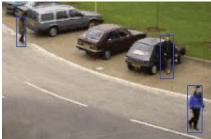
Figure 8.25 People detected using the histogram of oriented gradients technique. Image from the PETS 2000 dataset. The original image is reproduced by permission of Dr. James Ferryman, University of Reading
