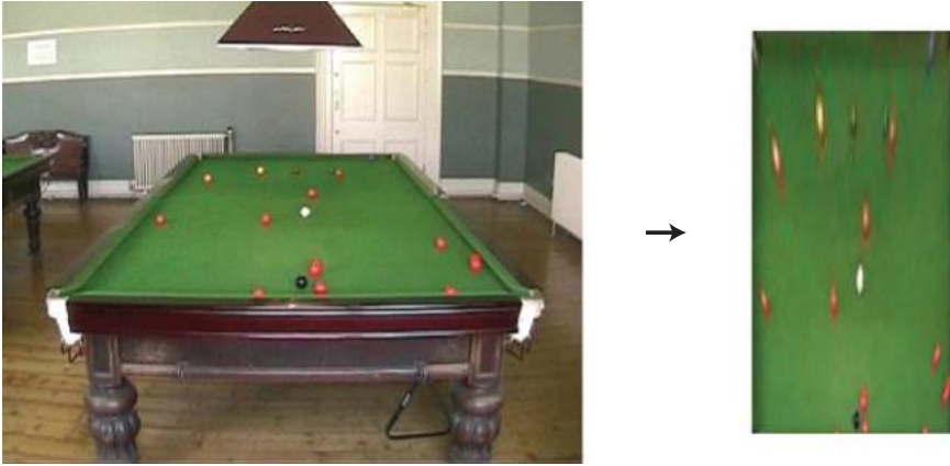
Figure 5.5 Perspective projection transformation to show the snooker table (left) from an aerial view-point (right). Note that the balls appear elongated in the corrected image because they sit above the plane for which the perspective transformation was computed
