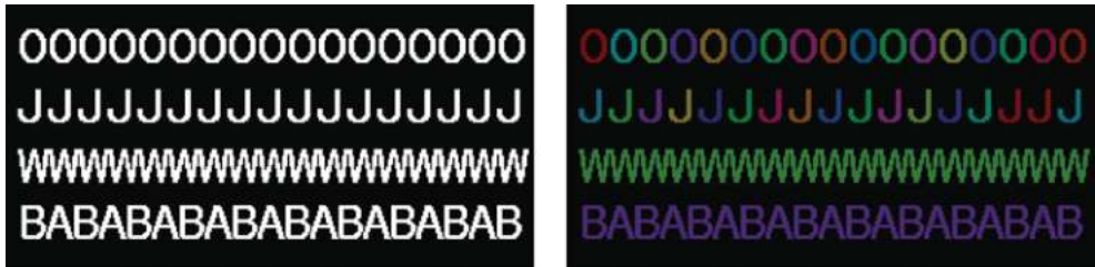
Figure 4.29 Application of Connected Components Algorithm using 8-adjacency on a test image
