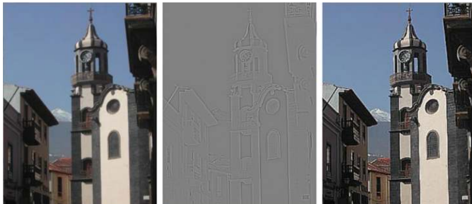
Figure 6.17 An original image (left), the second derivative (Laplacian) of that image (centre) and the sharpened image (right) which was computed by subtracting 0.3 times the second derivative from the original image
