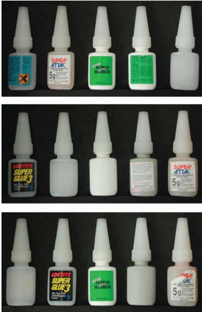
Figure 10.2 Sample images of bottles of glue are shown some without labels and some with crooked (or damaged labels). Note that these are not images from a real production line and in many cases the labels have been manually damaged/removed
