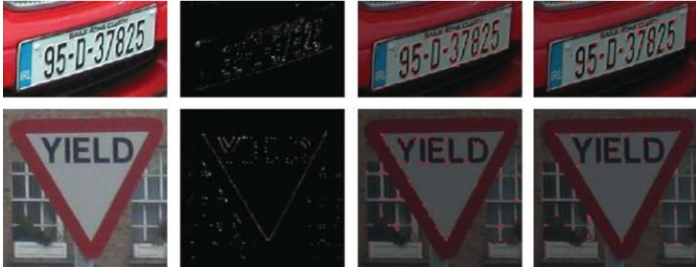
Figure 7.5 Two different images are shown (left) together with their Moravec cornerness maps (centre left), the Moravec corners detected (centre right) and the Harris corners detected (right)
