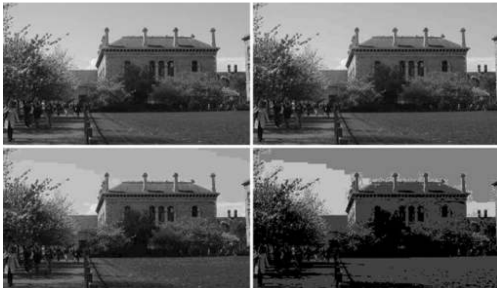
Figure 2.3 Four different quantizations of the same grey-scale image; top left 8 bits, top right 6 bits, bottom left 4 bits and bottom right 2 bits
