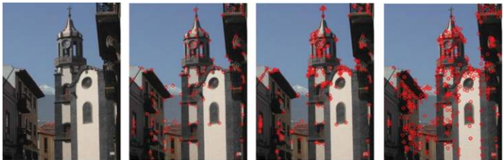
Figure 7.3 Corners/features detected from Harris (centre left), FAST (centre right), SIFT (right) from a greyscale version of the image on the left
