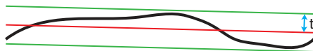
Figure 6.22 An edge contour (in black) together with a straight line approximation (in red). The bounds of the error are shown with green lines which are t pixels from the straight line approximation
