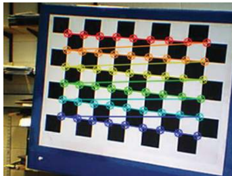
Figure 5.9 Image of a calibration grid with the located corners marked in various colours
