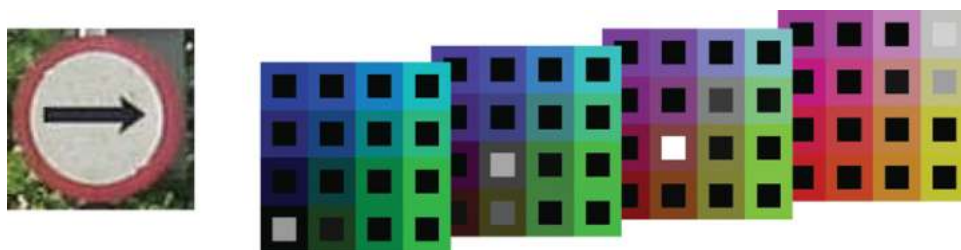
Figure 3.5 A 3D histogram (right) of the RGB channels from the colour image on the left. Note that the 0,0,0 point is shown on the front layer at the bottom left. The green axis goes from bottom left to bottom right of the front layer, the blue axis goes from bottom left to top left of the front layer and the red axis goes from bottom left of the front layer to bottom left of the bottommost layer. The average colour of each cell is shown as the border of the cell and the grey level intensity shown within in each cell indicates the relative number of pixels in each cell (black = 0, white = max). We can see several distinct peaks in the histogram for black points (front layer), grey points (2nd layer), red points (3rd layer) and white points (4th layer). The green image points are distributed across a few cells in the histogram
