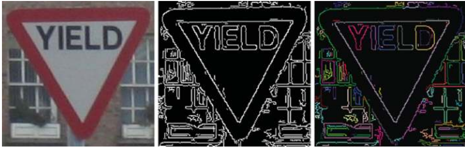
Figure 6.18 An image (left), the Canny edges detected (centre) and the extracted boundary chain codes shown in a variety of colours (right)
