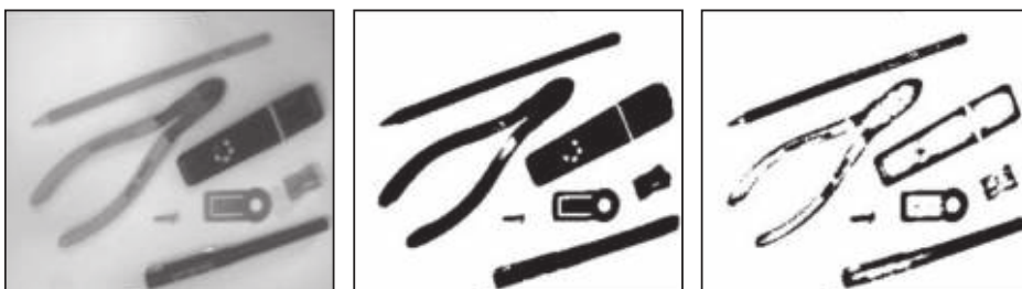
Figure 4.8 A 334×288 grey-scale image (left) which has significant variation in lighting across the image, together with two adaptively thresholded binary versions, computed using OpenCV's method, with a block size of 101×101 (middle) and 21×21 (right). An offset of 20 was used for both
