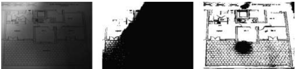
Figure 4.7 A grey-scale image (left) which has significant variation in lighting across the image, together with an optimally thresholded binary version (middle) and an adaptively thresholded binary version (right)
