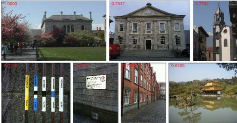
Figure 3.7 Best matching images (based on histogram comparison using a 3D HLS histogram with 2 bits on each channel; that is a 4 \times 4 \times 4 histogram). The reference image is the one on the top left (which gets a perfect matching score). The metrics shown in red are the correlation scores
