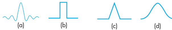
FIGURE 7.53 Display spots. (a) Ideal spot. (b) Rectangular approximation. (c) Piecewise-linear approximation. (d) Gaussian approximation.
