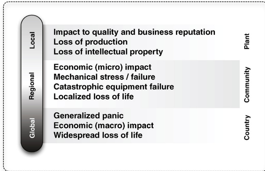
FIGURE 7.1 Consequences of a compromised industrial control system.
