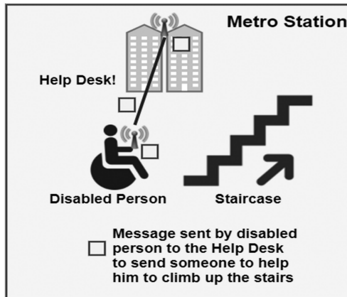
FIGURE 14.4 Delay-tolerant network deployed for disabled person.
