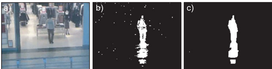
Figure 12.25 Background subtraction revisited. a) Original image. b) MAP solution of background subtraction model with independent pixels. The solution contains noise. c) MAP solution of background subtraction model with Markov random field prior. This smoothed solution has eliminated most of the noise.
