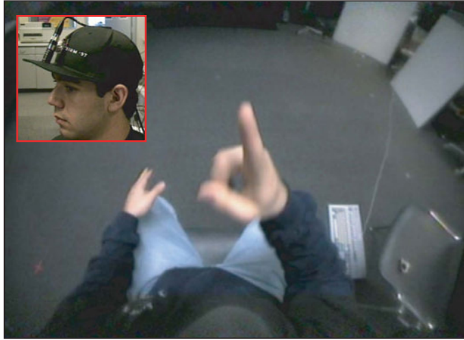
Figure 11.16 Gesture tracking from Starner et al. (1998). A camera was mounted on a baseball cap (inset) looking down at the users hands. The camera image (main figure) was used to track the hands in a HMM-based system that could accurately classify a 40-word lexicon and worked in real time. Each word was associated with four states in the HMM. The system was based on a compact description of the hand position and orientation within each frame. Adapted from Starner et al. (1998), ©1998 Springer.
