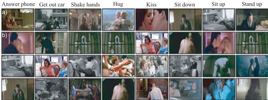
Figure 20.16 Action recognition in movie database of Laptev et al. (2008). a) Example true positives (correct detections), b) true negatives (action correctly identified as being absent), c) false positives (action classified as occurring but didn't) d) false negatives (action classified as not occurring but did). This type of real-world action classification task is still considered very challenging.
