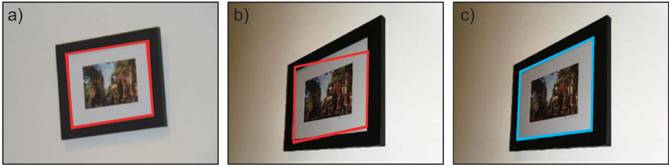
Figure 15.5 Approximating projection of a plane. a) A planar object viewed with a camera with a narrow field of view (long focal length) from a large distance. The depth variation within the object is small compared to the distance from the camera to the plane. Here, perspective distortion is small, and the relationship between points in the image and points on the surface is well approximated by an affine transformation. b) The same planar object viewed with a wide field of view (short focal length) from a short distance. The depth variation within the object is comparable to the average distance from the camera to the plane. An affine transformation cannot describe this situation well. c) However, a projective transformation (homography) captures the relationship between points on the surface and points in this image.
