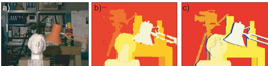
Figure 12.27 Stereo vision. a) One image of the original stereo pair. b) Disparity estimated using the method of Boykov et al. (1999). c) Ground truth disparity. Blue pixels indicate regions which are occluded in the second image and so do not have a valid match or disparity. The algorithm does not take account of this fact and produces noisy estimates in these regions. Adapted from Boykov et al. (1999).
