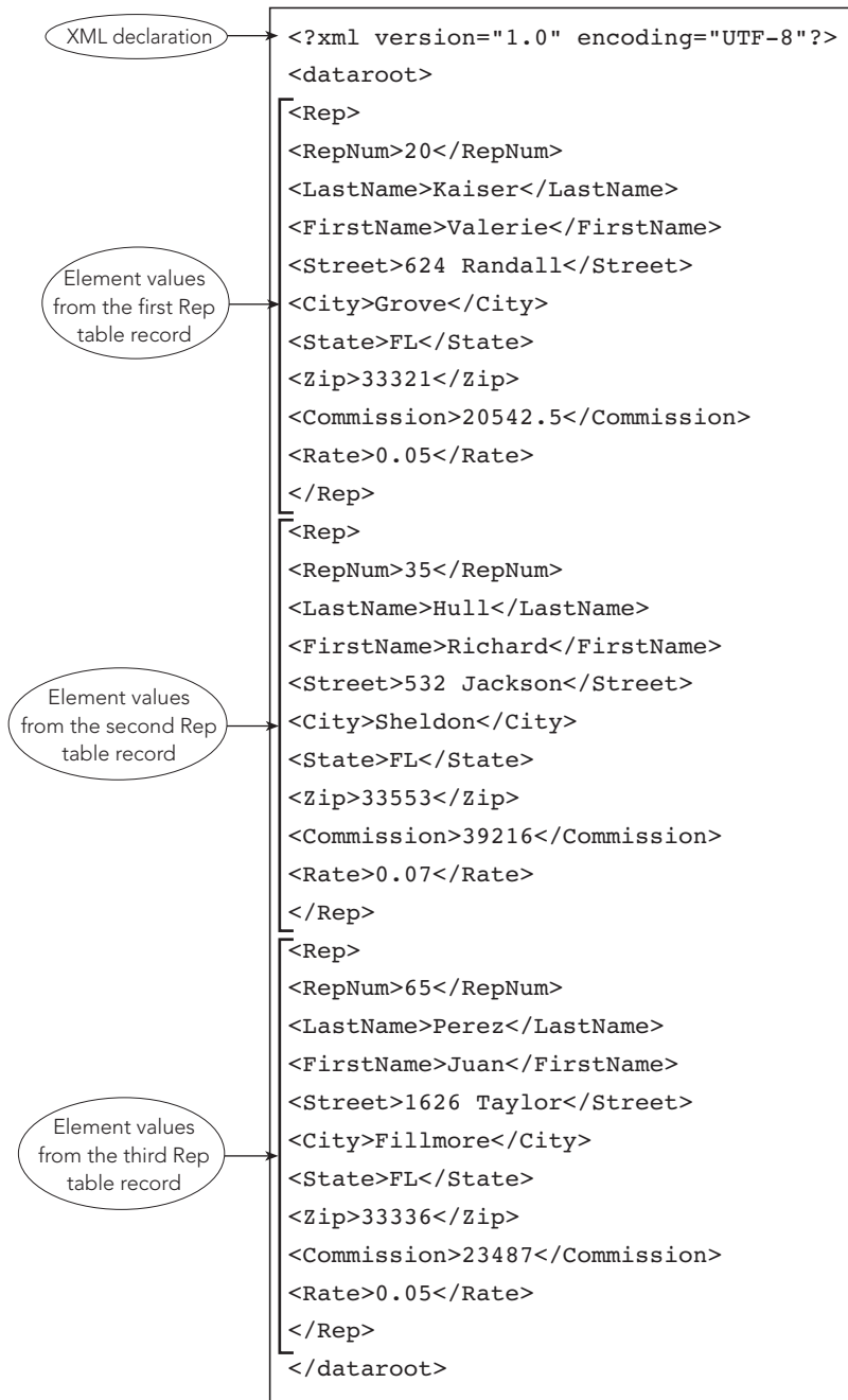
FIGURE 9-9 XML document created from the Rep table in the Premiere Products database
