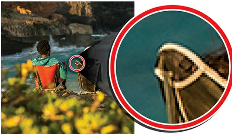
Example of a raster image and a zoomed-in portion to show the pixels.
