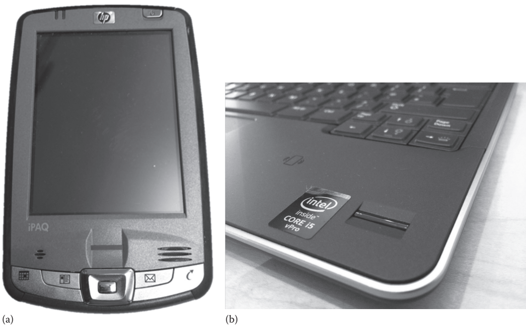
Figure 1.7 Fingerprint sensors provided as separate features on (a) a personal digital assistant and (b) a laptop personal computer.
