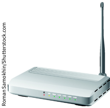
FIGURE 8.4 Wireless access point.
