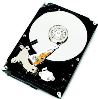
FIGURE TG 1.5 Traditional hard drives are less expensive, but solid-state drives are faster and are more reliable.
