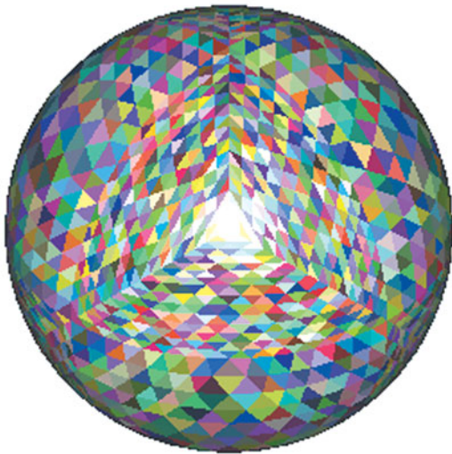
Color Plate 28 Sphere computed by recursive subdivision of tetrahedrons; triangle colors assigned randomly.
