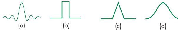
FIGURE D.13 Display spots. (a) Ideal spot. (b) Rectangular approximation. (c) Piecewise linear approximation. (d) Gaussian approximation.
