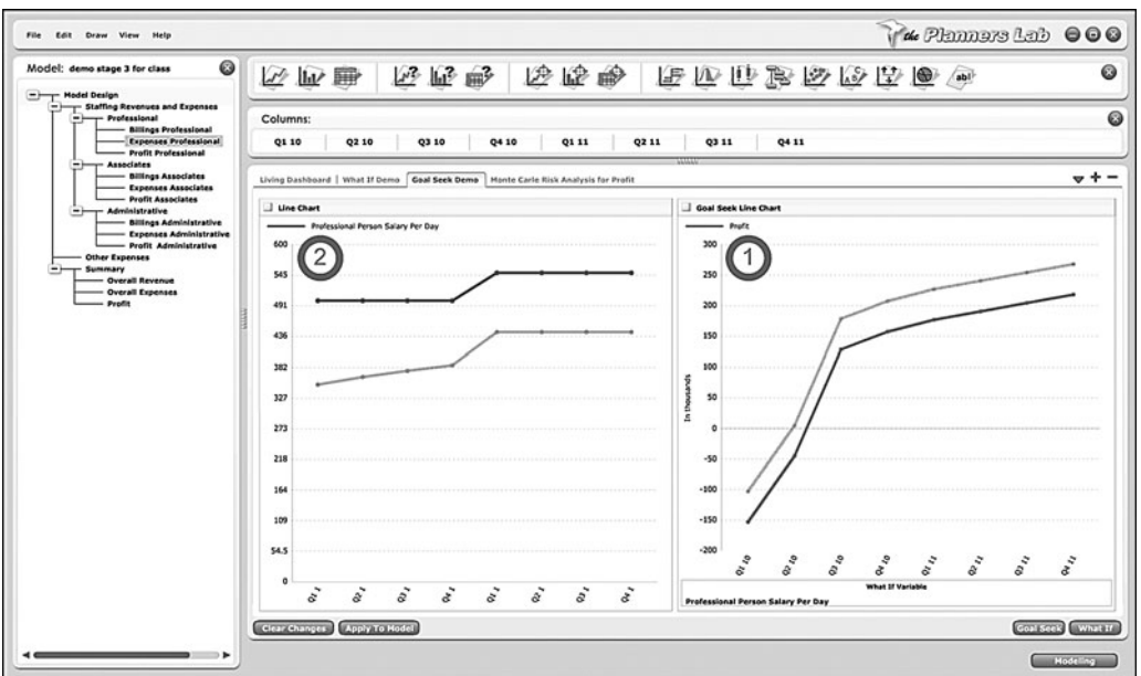
FIGURE 3.18 Goal Seeking to Determine Changes Needed in a What If Variable to Achieve Desired Result in a Goal Variable
