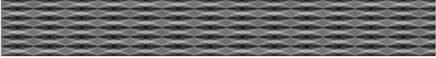
Figure 9.3: Simulated Talbot carpet: interference pattern behind grating G_1 travelling from left to right.
