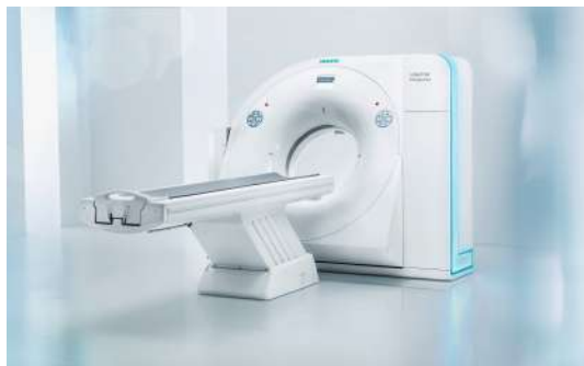
Figure 8.4: At the time of writing, a modern CT scanner can acquire up to 128 image slices in parallel. Image courtesy of Siemens Healthineers AG.
