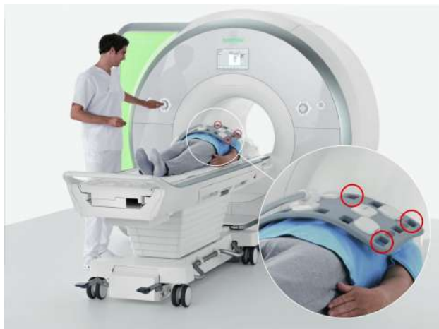
Figure 6.11: Parallel imaging uses local receiver coils placed around the patient which capture the signal from multiple positions, allowing for a reduction of acquisition time. The coils are embedded in the table as well as in the flexible coil on top of the patient’s chest, in this case an 18-element body coil where individual coil elements are arranged in 6 columns and 3 rows. Three individual coil elements are exemplarily indicated by the red circles. Image courtesy of Siemens Healthineers AG.
