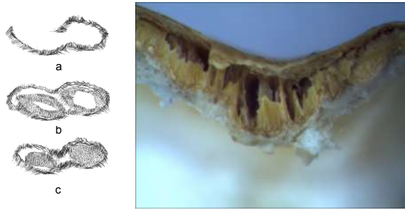
Figure 1.4: An X-ray dark-field setup can be used to reconstruct the orientation of fibers that are smaller than the detector resolution. The image on the left shows the reconstructed fiber orientation in different layers of a peanut. The image on the right shows a microscopic visualization of the waist of the peanut (picture courtesy of ECAP Erlangen).
