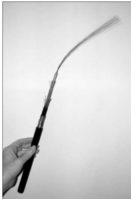
Figure 3-7 A fiber-optic cable with multiple strands of fiber
