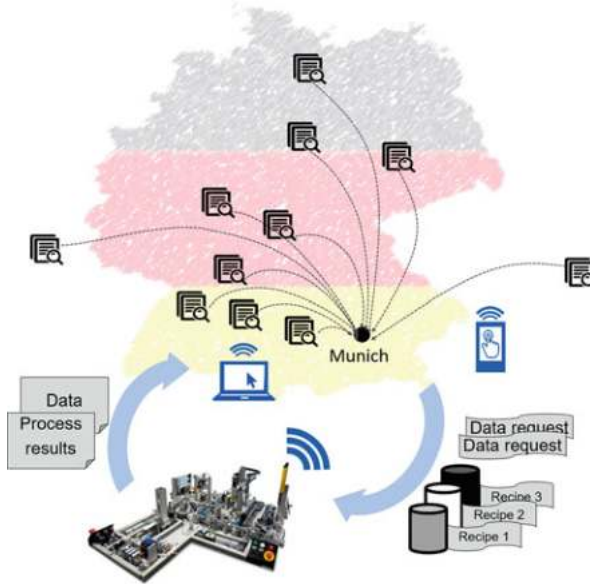
Fig. 12.23 Remote connection of the xPPU Industry 4.0 interface
