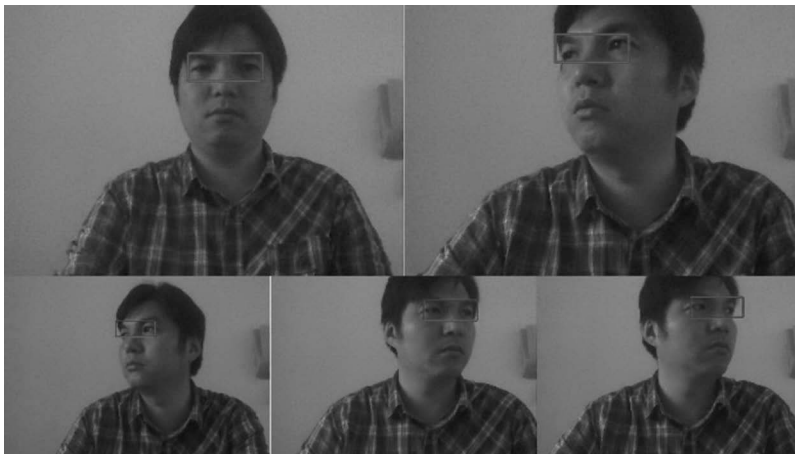
Figure 3.16 Eye location by using the Haar-like feature in a real-time video stream.
