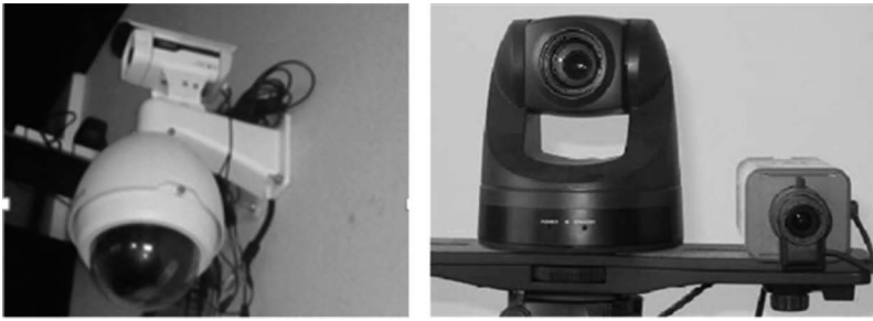
Figure 3.24 Dual-camera configuration in identity verification system.
