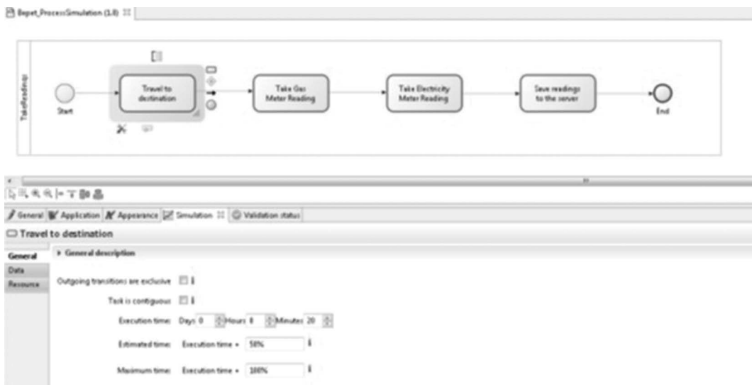
Figure 9.10 Simulation parameters for meter reading.
