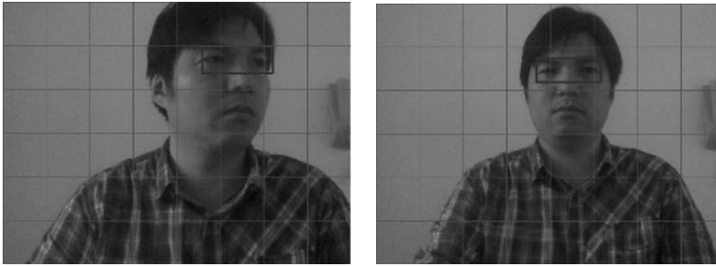
Figure 3.18 Illustration of eye location and the grid of subimages.
