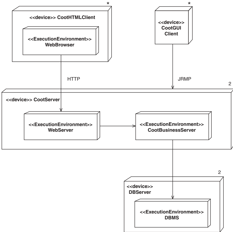
Figure 9.9: A more detailed deployment diagram for iCoot
