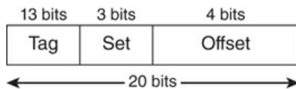
FIGURE 6.16 4-Way Set-Associative Mapped Memory Format for Example 6.6
