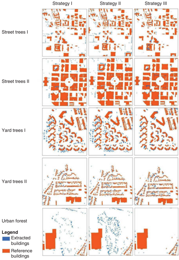
FIGURE 6.10 Nonbuilding pixels mislabeled as buildings in the three strategies of building extraction (blue pixels not covered by orange ones).
