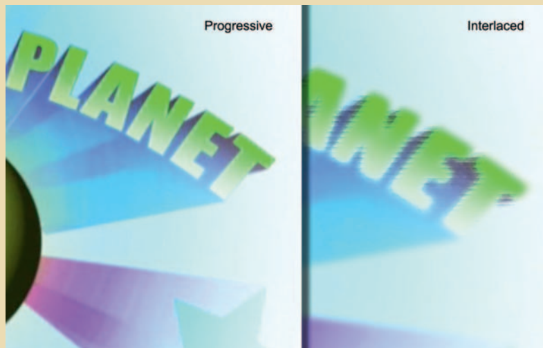
Figure 13.12 720p footage has a frame size of 1280 \times 720 and is progressive scan; 1080i footage is interlaced with a frame size of 1920 \times 1080 .
