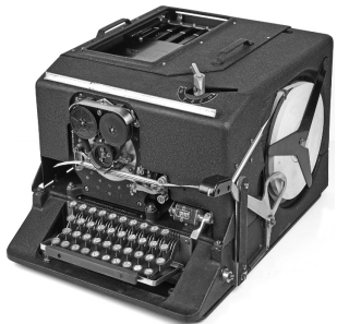
Figure 12.9: SIGABA (Reproduced with permission from www.cryptomuseum.com )
