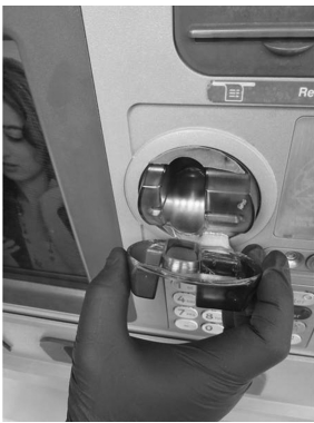
Figure 02.4: ATM skimmer (Reproduced with permission from Aurora Police Department)
