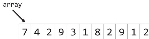
Figure A.1: How an array is stored in memory with most programming languages
