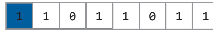
Figure D.5: Adding one completes the 2’s complement where the first bit is the sign (+/-)
