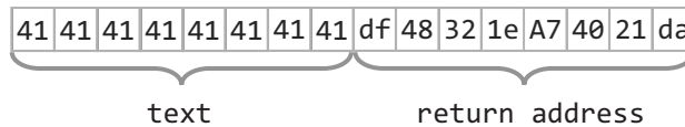
Figure 07.11: Malicious input placed in a vulnerable stack buffer to achieve Stack Smashing. Notice the address of dangerous() in the return buffer.
