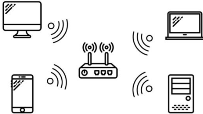
Figure 1: Computing devices contain wireless adapters which communicate with an access point (shown at center).
