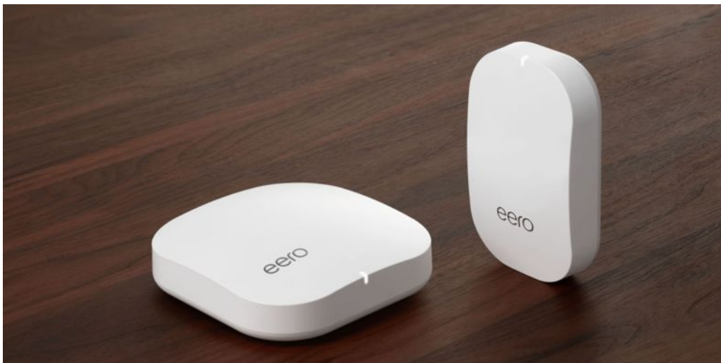
Figure 13: Startup eero offers two models of mesh nodes, the eero (left) and the Beacon.
