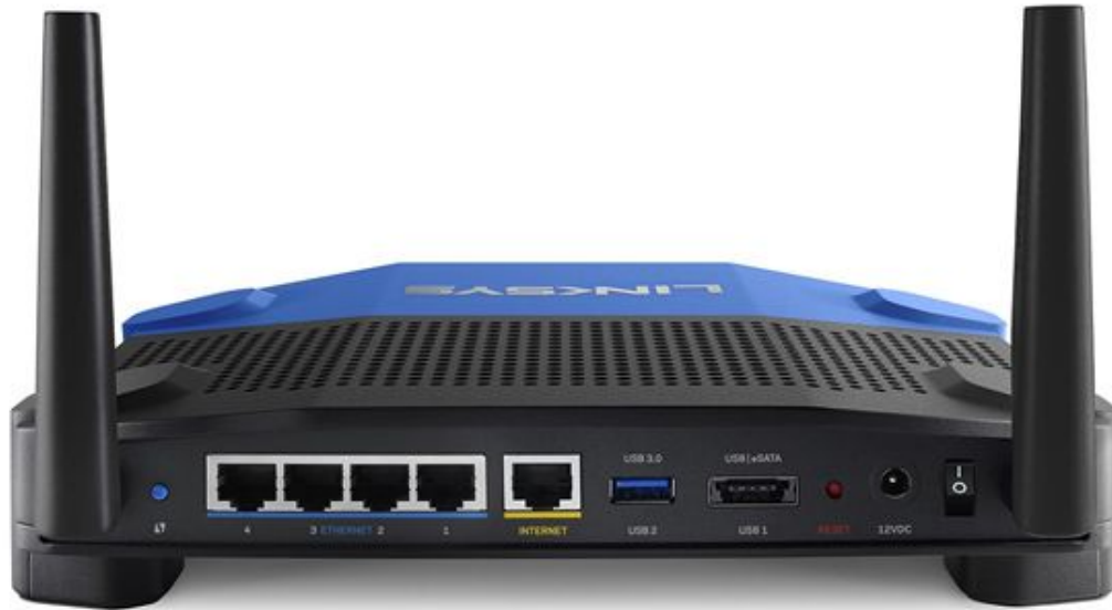
Figure 2: Gateways feature built-in Ethernet switches, as you see here at the left of this Linksys WRT1200AC.
