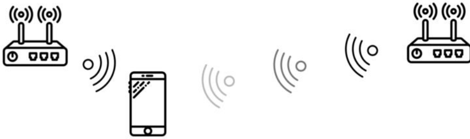
Figure 3: When there are multiple access points in a network, a wireless device will switch to the one with the stronger signal.
