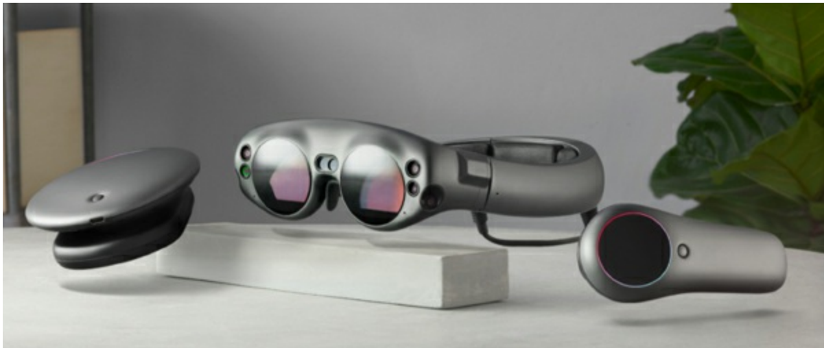
Figure 12.16. The Magic Leap One MR kit: Processing unit (left), headset (center), and controller (right)
