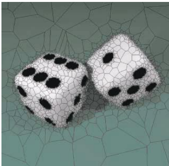
Plate XVI. Nonuniform representation: Voronoi cells (2,000 samples). (Reprinted from [Darsa et al. 98], with permission from Elsevier. See page 240.)
