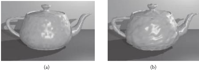
Figure 16.23. A deformed Utah teapot using the same texture for (a) bump and (b) displacement mappings. (From [Wolfe 97], ©Rosalee Wolfe. Used with permission. See Color Plate XXXIV.)
