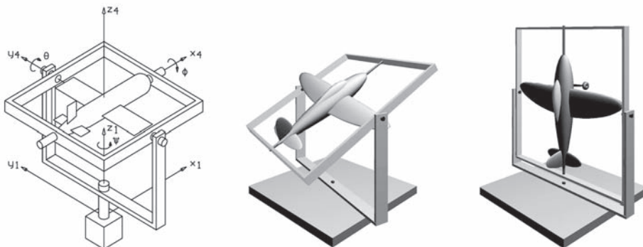
Figure 4.4. Gimbal lock phenomenon. Schematic illustration for rotating an aircraft: by the yaw angle \Psi about the z -axis, by the pitch angle \theta about the y -axis and the roll angle \varphi about the x -axis (left); rotating the aircraft (middle); the yaw gimbal rotates 90 degrees and the aircraft is free to move about the z -axis (right). (Figures courtesy of Gernot Hoffmann [Hoffmann 03].)
