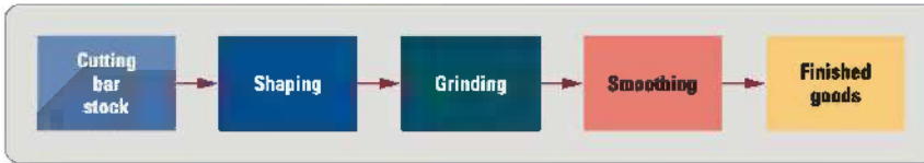
EXHIBIT 4-23 Sequence of Operations for Drill Bit Production
