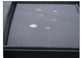
Figure 26.15: Fresnel's law in action: The coins are easily visible from overhead, but are obscured by sky reflections when seen at a diagonal.
