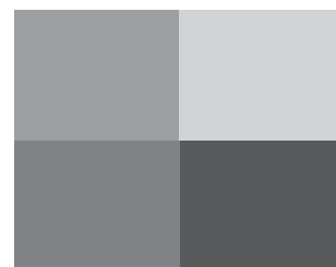
Figure 18.19: The values in a 2 \times 2 grayscale image are convolved with a box function to get a piecewise constant function on a 2 \times 2 square.
