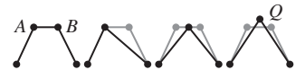
Figure 8.15: Different geometric choices for an edge collapse in 2D. The edge AB is collapsed; one can (a) place the collapsed vertex at A for computational simplicity, (b) at the midpoint of the segment AB , or (c) at a point Q that minimizes the maximum (or average) distance from every old mesh point to the nearest new mesh point. Other goals are possible as well.
