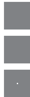
Figure 5.2: Three 41 \times 41 -pixel images. The top image has all pixel values 118; the middle has all pixel values 128; the bottom has all pixel values 128, except the center, which is 255. The L^2 distances from the top image to each of the others are approximately equal, but this does not match our own understanding of “sameness.”
