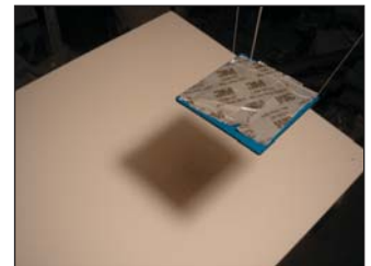
Figure 18.20: The square occluder casts a shadow with both umbra and penumbra when illuminated by a round light source.
