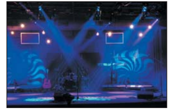
Figure 14.33: A photograph of spiral patterns created by real gobos in spotlights (Credit: R. Gino Santa Maria/Shutterstock.com).
