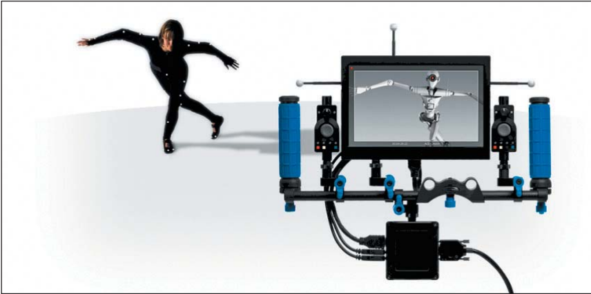
Figure 35.4: Motion capture systems, such as the InsightVCS system pictured, record the three-dimensional motion of a real actor and then apply those motions to avatars in the virtual scene. (Courtesy of OptiTrack.)
