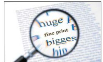
Figure 14.11: The rainbowlike edges on the objects in this photograph are caused by chromatic aberration in the camera's lens. Different frequencies of light refract at different angles, so the resultant colors shift in the image plane. High-quality cameras use multiple lenses to compensate for this effect. (Credit: Corepics VOF/Shutterstock)
