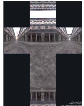
Figure 33.4: An environment map of the Uffizi, specified by six texture maps, one each for the top, bottom, and four vertical sides of a cube, displayed here in a cross-layout. (Courtesy of Paul Debevec. Photographs used with permission. ©2012 University of Southern California, Institute for Creative Technologies.)
