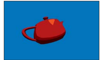
Figure 33.6: Toon shading using a vertex shader; notice the sharp corners of the highlight area.
