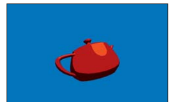
Figure 33.7: Toon shading using a fragment shader. Notice the smooth boundary between the shades of red.
