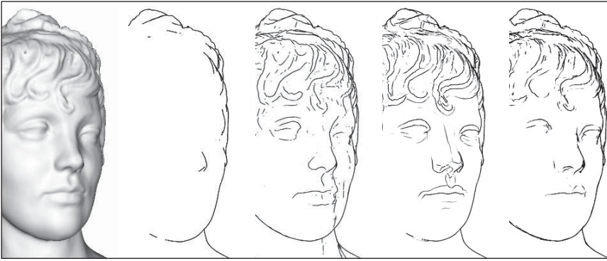
Figure 34.18: Shaded view, contours, suggestive contours, ridges and valleys, and apparent ridges for a single model. Courtesy of Tilke Judd and Frédo Durand, ©2007 ACM, Inc. Reprinted by permission.)
