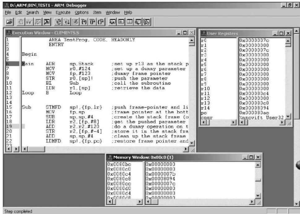
(c) Snapshot of the register and memory state at the end of the program
