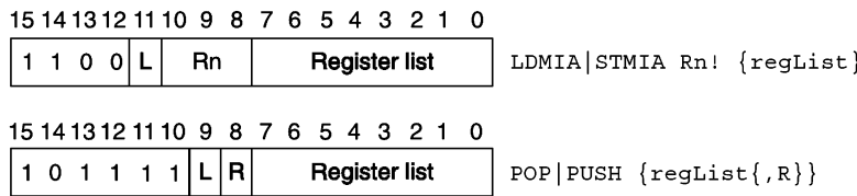
FIGURE 4.31 Encoding the Thumb-mode multiple register transfer instructions
