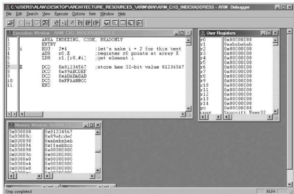
FIGURE 3.36 Example of the use of pre-indexed register indirect addressing
