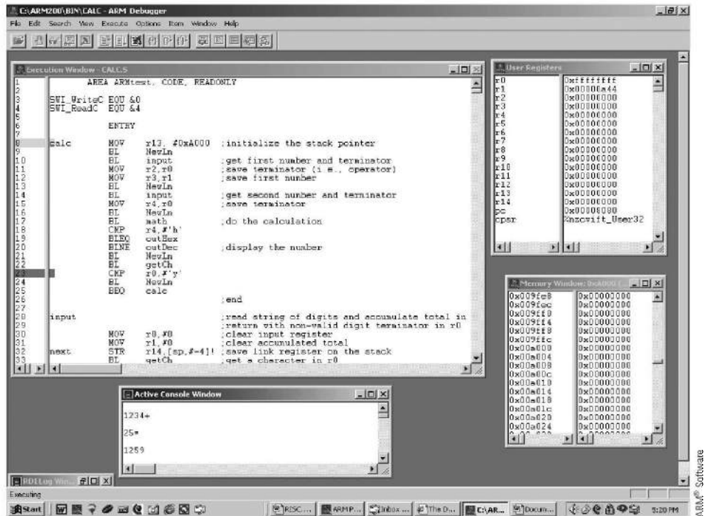
FIGURE 3.13 Snapshot of the ARM debugger window
