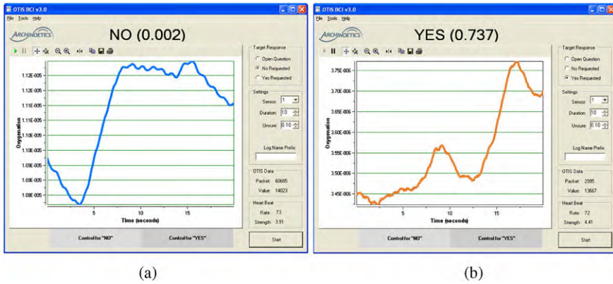
Fig. 8.4 The OTIS BCI application graphs oxygenation data in real-time and then provides the state determination at the end of the trial. The “NO” screenshot on the left shows the hemodynamic response while the subject performs the active task followed by the inactive task (the order is reversed in the “YES” screenshot on the right). The scores at the top reflect the confidence in the yes/no determination, where 0 is a strong “NO”, 1 is a strong “YES”, and 0.5 is inconclusive
