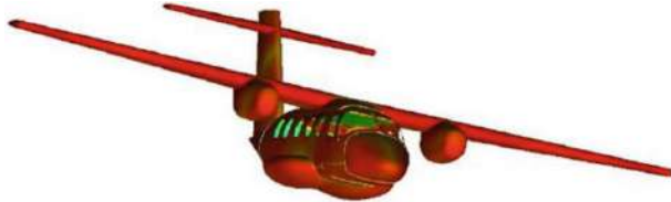
Fig. 1. Surface currents on an aircraft model from a boundary element simulation with around 2 million unknowns.
