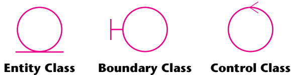
FIGURE 13.1 UML stereotypes (extensions of UML) for representing an entity class, a boundary class, and a control class.
