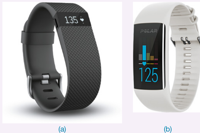
Figure 14.1 Devices for monitoring activity and heart rate (a) Fitbit Charge and (b) Polar A370
