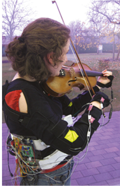
Figure 7.21 The MusicJacket with embedded actuators that nudge the player to move their arm up to be in the correct position
