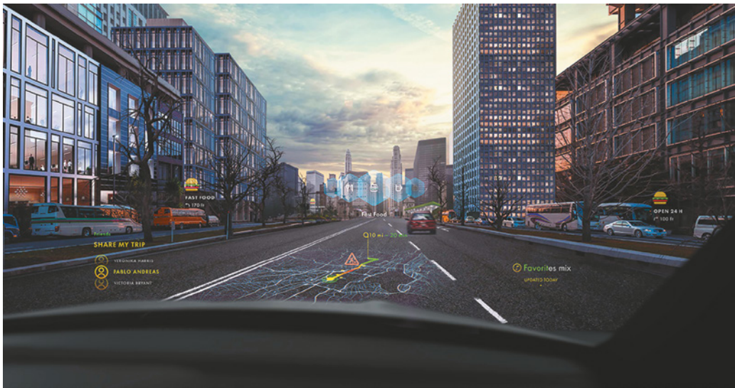
Figure 7.27 Augmented reality overlay used on a car windshield
