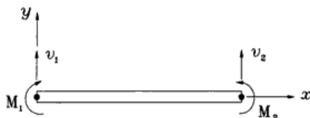
Figure 8.4.1 Linear Mixed Beam Element
