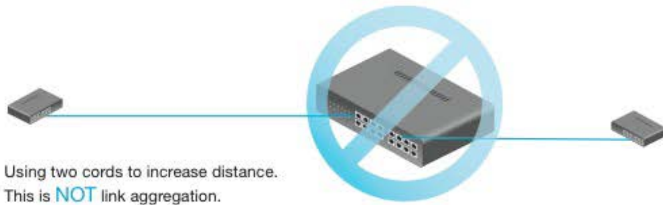
FIGURE 5-18 Link Aggregation Increases Speed, not Distance
