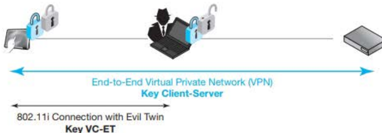
FIGURE 7-12 Defeating an Evil Twin Attack by Using a Virtual Private Network (VPN)
