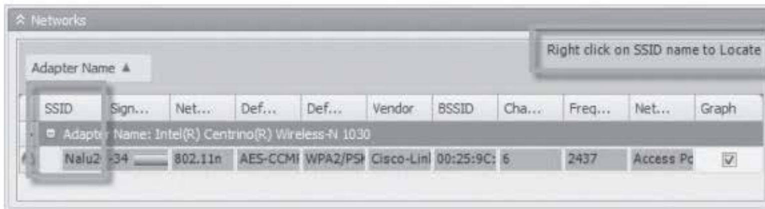
FIGURE 6a-4 Locating an Access Point
