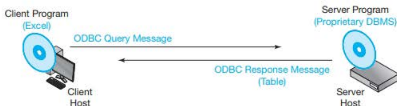
FIGURE 1-10 Not Always Browsers and Webservers: Excel Querying a Proprietary Database Management System (DBMS) Using the Open Database Connectivity Protocol (ODBC)
