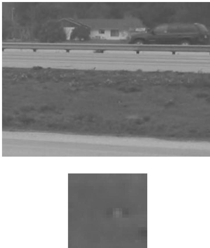
Figure 3.7 Hot pixel in an image (top) and its closeup (bottom). Because the hot pixel had a red filter in front of it, the hot pixel appears red. Note the spread of the red color due to demosaicking and other in-camera processing. For a color version of this figure, see Plate 3.
