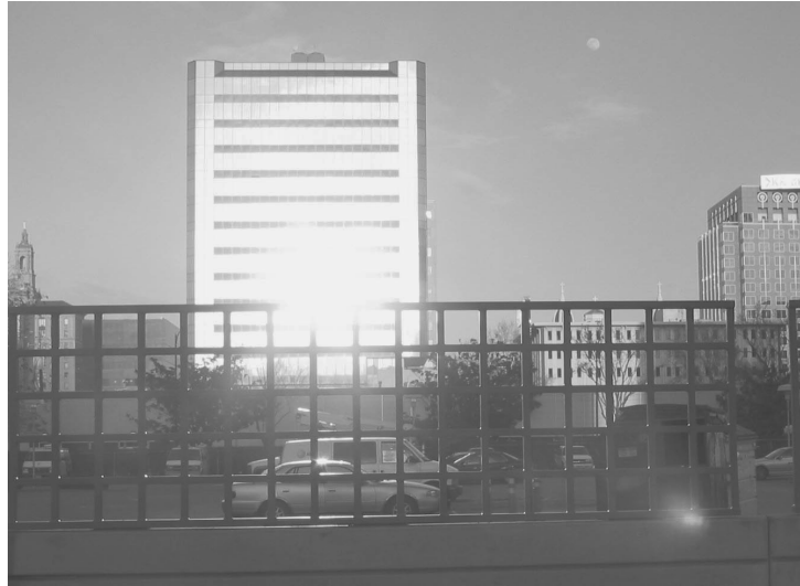
Figure 3.8 Blooming artifacts due to overexposure. Also, notice the green artifact in the lower right corner caused by multiple reflections of light in camera optics. A color version of this figure is displayed in Plate 4.
