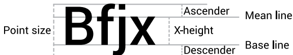
Figure 4-6 An illustration with the Roboto font showing how a font size is measured
