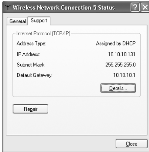
Figure 13.16 Windows XP's Wireless Network Connection status showing a good DHCP-issued address, indicating a successful connection to a local access point.
