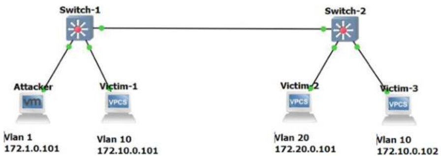
Fig. 6.17 A scenario with pre-configured VLANs and default settings
