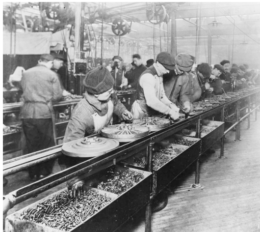
Fig. 3.1 Workers on the first moving assembly line put together magnetos and flywheels for Ford cars. Taken by unknown photographer in 1913 2 .
