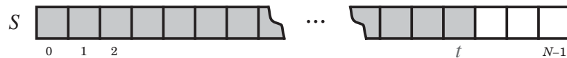
Figure 2.2: Implementing a stack with an array S . The top element is in cell S[t] .
