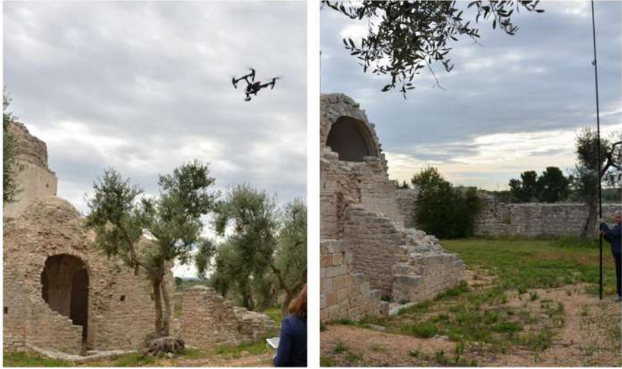
Fig. 8. The 3D model was obtained using SfM software by means of images by a camera mounted on an unmanned aerial vehicle (left) and by a multi-camera system ad hoc-developed (right).
