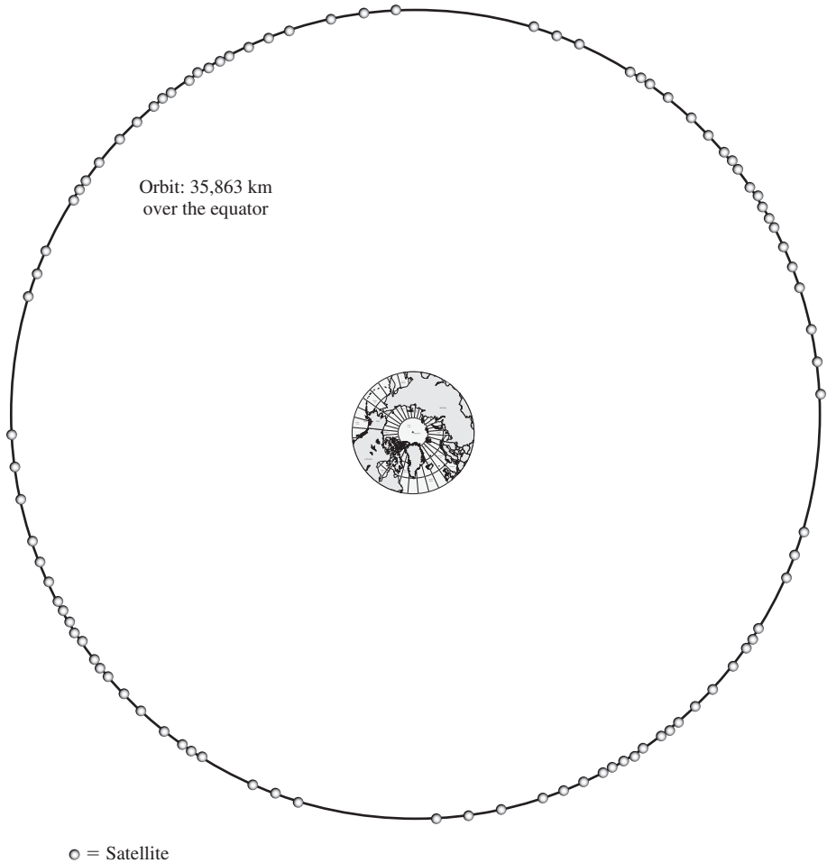
Figure 17.11 Geostationary Earth Orbit (GEO)
