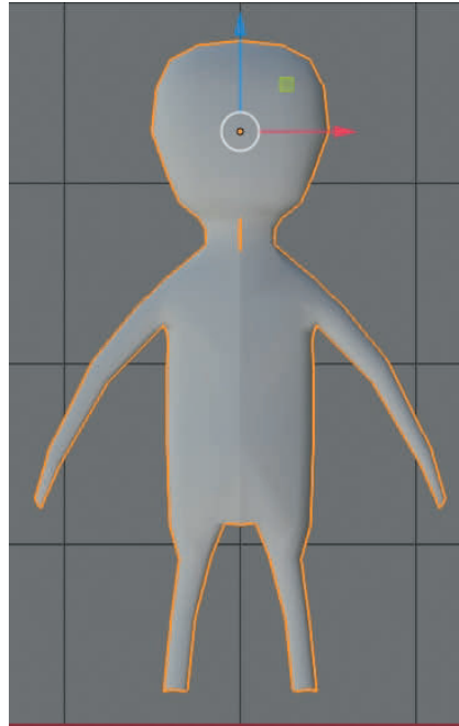
In Object Mode set Shading to Smooth and Apply the Mirror Modifier.
