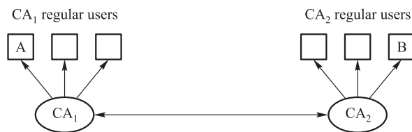
Figure 3.4 A CA network consisting of two CAs that can verify each other's public key
