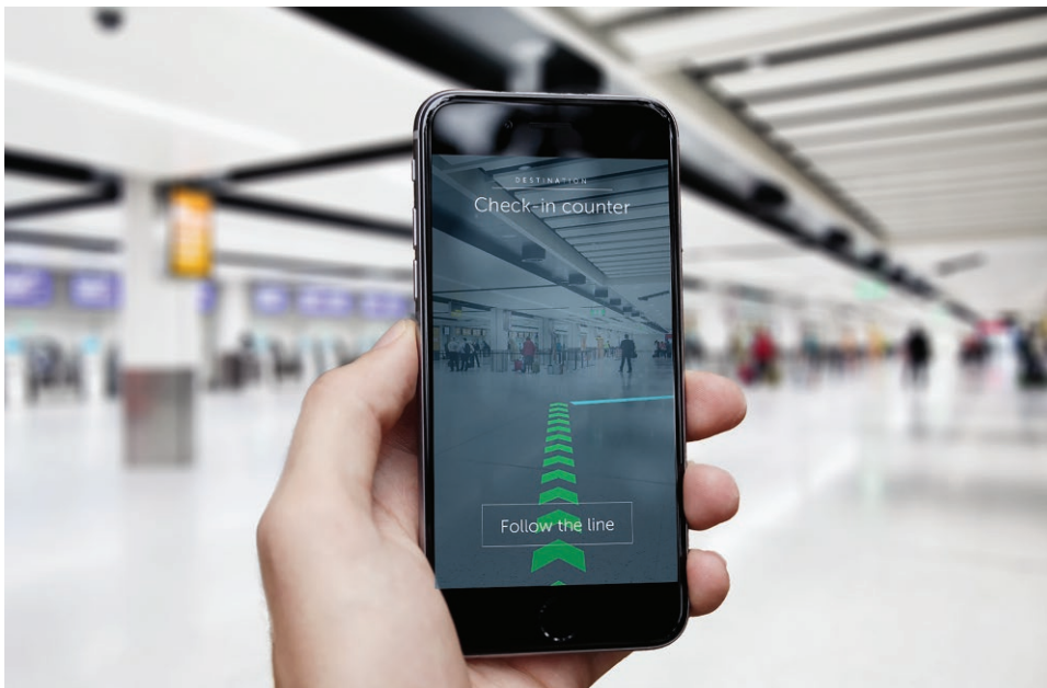
Figure 7.7 Gatwick Airport augmented reality wayfinding app using beacons
