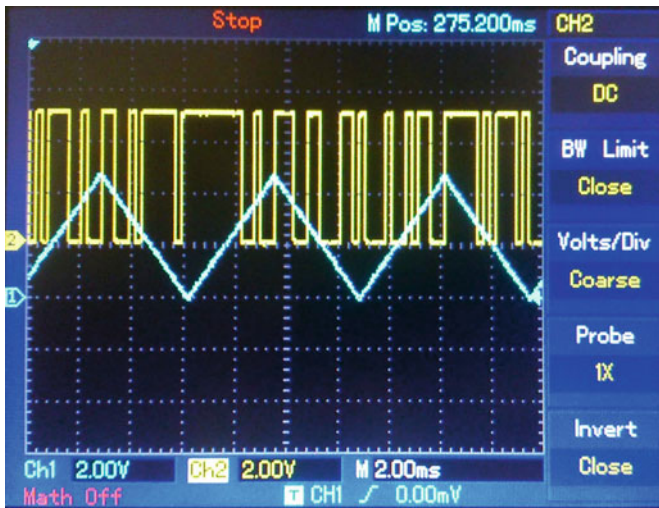
Fig. 15 160Hz triangular wave message. Blue: sent message. Yellow: encrypted message
