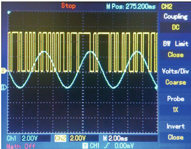
Fig. 11 160 Hz sine wave message. Blue: sent message. Yellow: key signal
