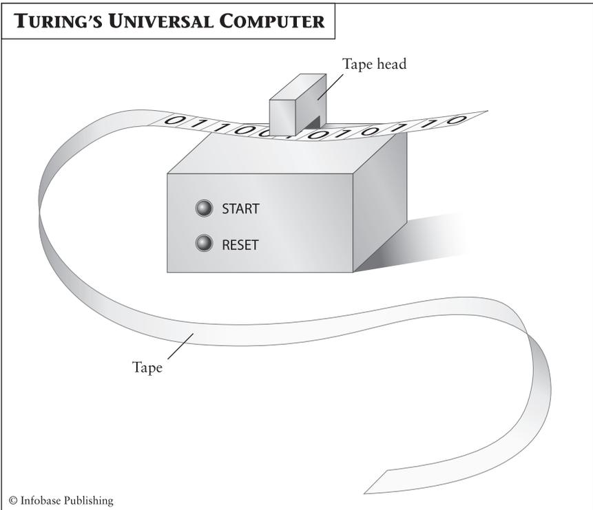
*The conceptual Turing Machine consists of an endless tape that can be moved back and forth while recording or erasing symbols.*
