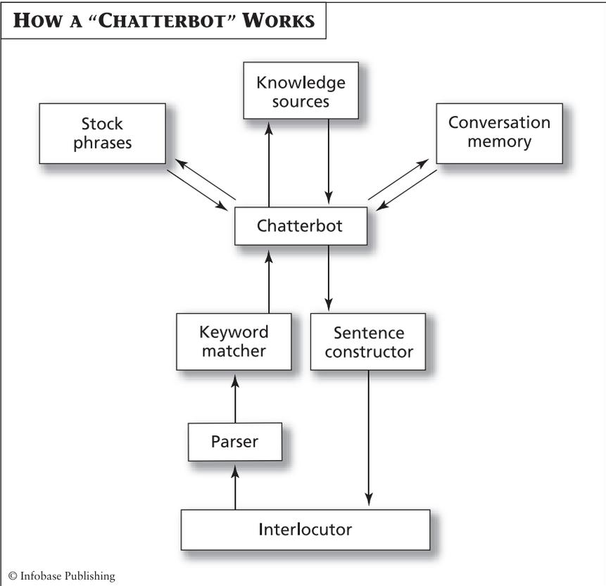
*This schematic shows how a typical “chatterbot” processes the input from the human (interlocutor) and constructs a reply. Note that more sophisticated chatterbots enhance the illusion of true conversation by remembering and returning to previously discussed topics.*
