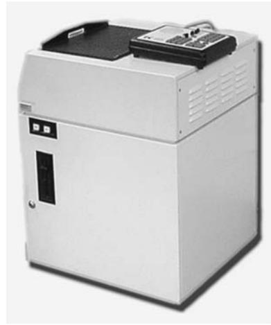
*Kurzweil’s first reading machine was about the size and shape of an office copier. Since it scanned text with a copier-like mechanism, perhaps this was not so surprising. (Kurzweil Technologies)*
