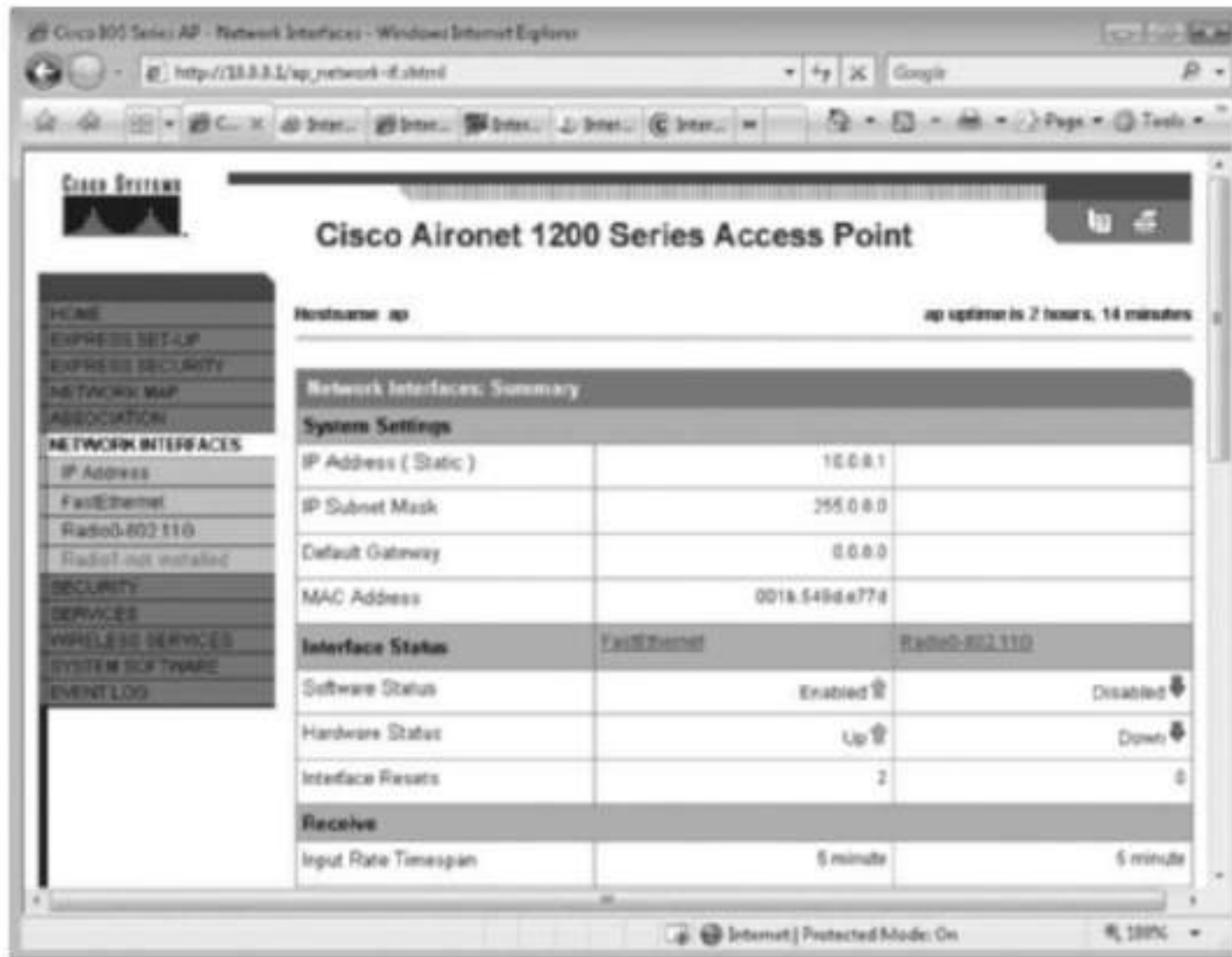
Figure 9-9 Status of the Ethernet and radio interfaces
