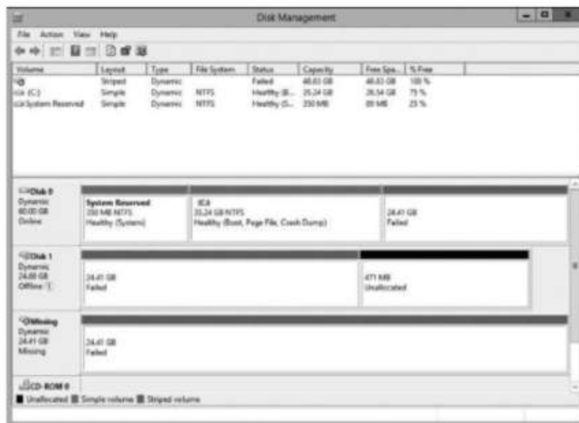
Figure 13-3 Failed striped volume
